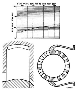
Fig. 16-13. Curtis' Model Test on Cross Scavenging.
