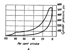
Fig. 10-2. Typical Indicator Diagrams (a) Four-Stroke Cycle, and (b) Two-Stroke Cycle Diesel Engines.
