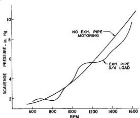
Fig. 16-21. Scavenge Pressure vs. Rpm of a Three-Cylinder GM 3-71 Engine. The exhaust system mounted shows favorable tuning from 1300 to 1500 rpm and unfavorable tuning around 1100 rpm. (Penn State Diesel Laboratory.)
