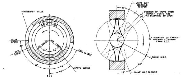
Fig. 9-5. Port Timing with Cooper-Bessemer Supercharge Valve. (By permission of Cooper-Bessemer Corp.)
