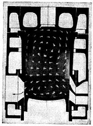
Fig. 5-7. Flat Scavenge with a Counterclockwise Swirl on the Bottom and a Clockwise Swirl Above It.
