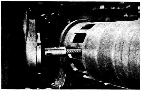
Fig. 6-7. Milling of Ports in Cylinder Liner. (By permission from F. Sass, Kompressorlose Dieselmaschinen. Copyright, 1929 by Julius Springer in Berlin.)
