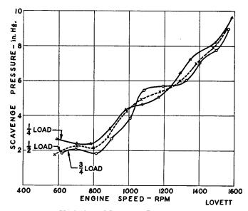
Fig. 16-22. Variation of Scavenge Pressure with Speed and Load. General Motors 3-71 Engine. (Penn State Diesel Laboratory.)
