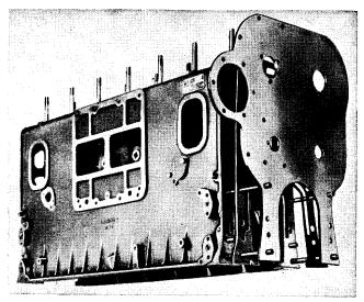
Fig. 17-3. GM 6-71 Cylinder Block. Rear end plate in front.
