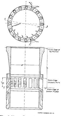
Fig. 9-13. Port Arrangement of Nordberg 21 in. × 31 in. Engine. (By permission of Nordberg Manufacturing Company.)
