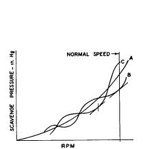
Fig. 16-20. Scavenge Pressure vs. Rpm Shows Exhaust Tuning or Lack of It.
