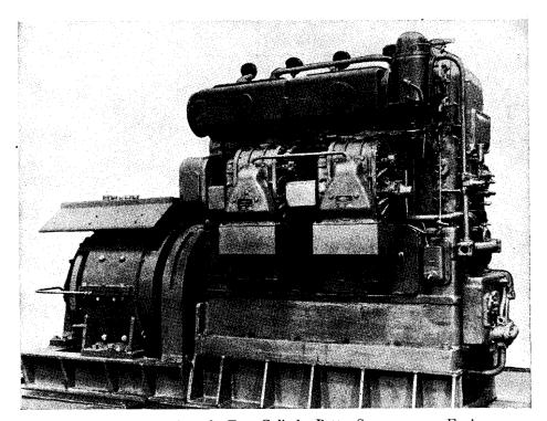
Fig. 13-7. Back View of a Four-Cylinder Petter Superscavenge Engine.
