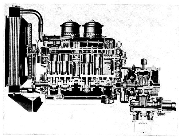
Fig. 17-12. Lubrication Passages.
