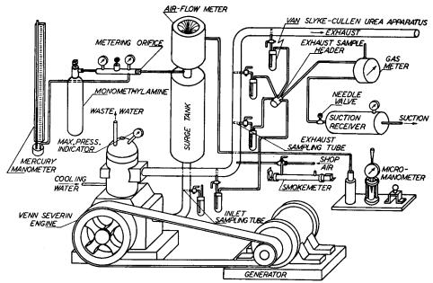
Fig. 16-6. Setup for Testing Engine Scavenge with the Tracer Gas Method. (Penn State Diesel Laboratory.)
