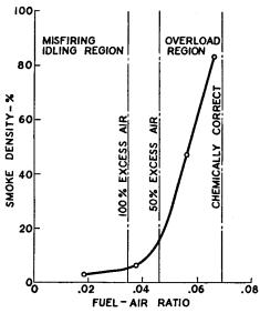
Fig. 16-29. Smoke Density Plotted against Load Indicates a "Hot" Engine. Compression ratio, 18:1. (Penn State Diesel Laboratory.)
