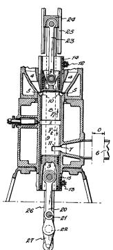
Fig. 13-10. U. S. Patent No. 2,113,480, M. Kadenacy. lead is so varied that the desired timing is obtained for varying engine speeds.
