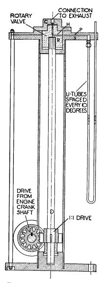
Fig. 16-24. Schematic Drawing of Penn State Rotary-Valve Low-Pressure Indicator.
