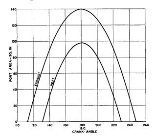
Fig. 14-1. Preliminary Port Area Diagram.
