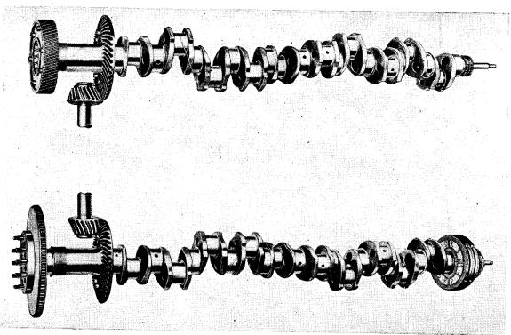
Fig. 17-24. Upper and Lower Crankshafts.
