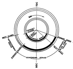
Fig. 2-2. Timing Diagrams. Inner diagram, symmetrical scavenge. Outer diagram, unsymmetrical scavenge.
