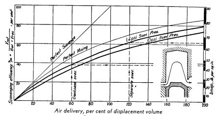
Fig. 5-8. Scavenging Efficiency of Cross Scavenging. Scale on right shows the bmep attainable with 60% excess air, 100% relative charge, and 0.5 lb per hp-hr fuel consumption. 70% of the bmep reading represents fair output for symmetrically scavenged engines and 100% for the supercharged engines.
