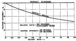
Fig. 3-4. Trapping Efficiency vs Delivery Ratio.
