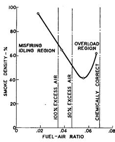
Fig. 16-28. Smoke Density Plotted against Load Indicates a "Cold" Engine. Compression ratio, 12:1. (Penn State Diesel Laboratory.)
