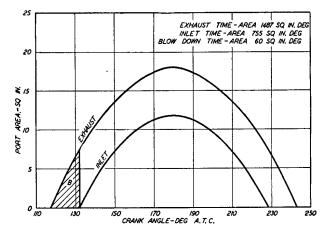
Fig. 8-7. Porting Diagram of Venn-Severin Engine. 10.5 in. bore; 12 in. stroke; 425 rpm.
