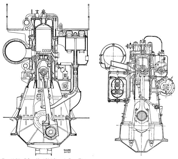
Fig. 12-15. Sulzer  $22 \times 39.4$  in., 165 Rpm Engine with Welded Steel Exhaust Header.
