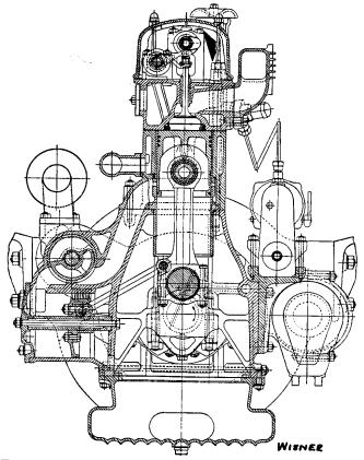
Fig. 11-5. Ricardo's 63/3 Experimental Engine. (R. Wisner, *High Speed Two-Stroke Compression-Ignition Engine*. The Institute of Automobile Engineers, June, 1944.)
