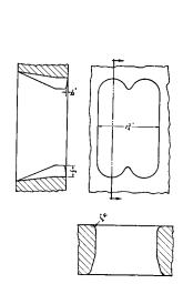
**Fig. 6-3.** Gothic Exhaust Port. Note relieved lip and rounding of side edges.
