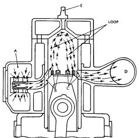
Fig. 12-17. Crossley-Carter Loop Scavenged Engine. A. Air under pressure in air manifold. B. Intake Ports. C. Exhaust Ports. D. Exhaust Manifold. E. Fuel Injector. (H. D. Carter, "The Loop-Scavenged Diesel Engine," *Proc. Inst. M. E.*, 154, No. 4, 1946.)
