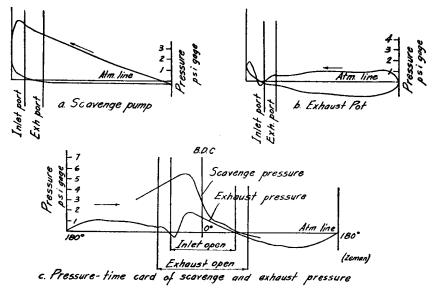
Fig. 16-18. Weak-Spring Diagrams with a Properly Functioning Exhaust System. 12.6 in. bore, 14.6 in. stroke. 309 rpm; exhaust pipe 5.9 in. dia., 256 in. long; exhaust pot 8.7 cu. ft. (J. Zeman, Zweitakt Dieselmaschinen. Copyright, 1935, by Julius Springer in Vienna.)
