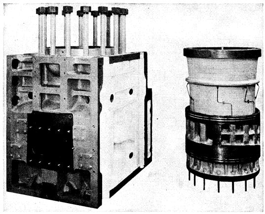
Fig. 17-32. Nordberg Cylinder and Liner.
