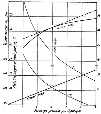
Fig. 7-9. Determining the Optimum Scavenge Pressure for Engine Shown in Fig. 7-8.
