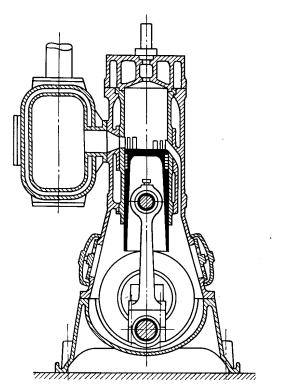
Fig. 2-3. Crankcase-Scavenged Engine (Sulzer).
