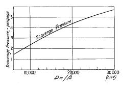
Fig. 7-1. Selection of Scavenge Pressure. D= Cylinder diameter in inches, n= Revolutions per minute,  $\beta=$  The ratio of the inlet port width (square to the flow) to the circumference  $=b_i/D\pi$ .
