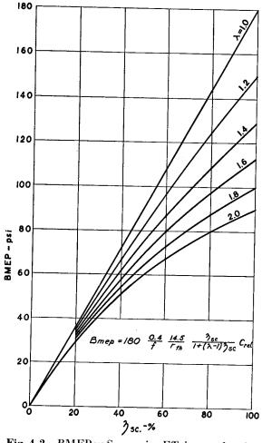
Fig. 4-2. BMEP vs Scavenging Efficiency. f = 0.4 lb per bhp-hr,  $r_{th} = 14.5$ ,  $C_{rel} = 1$ .
