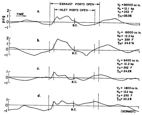
Fig. 12-9. Indicator Diagrams Showing the Effect of Size of Expansion Chamber. Pressure fluctuations in the exhaust near the exhaust ports.
