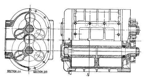
Fig. 11-9. Typical Three-Lobe Blower, Made by B-W Superchargers, Inc. (By permission of B-W Superchargers, Inc.)
