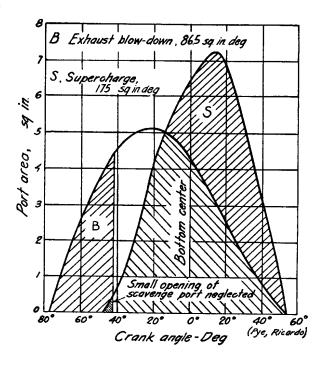
Fig. 9-10. Porting Diagram, Ricardo Sleeve Valve Diesel Engine. (D. R. Pye, *The Internal Combustion Engine*, Oxford at the Clarendon Press, 1934.)
