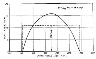
Fig. 9-16. Reduced Time-Area Diagram of Fairbanks-Morse Opposed-Piston Engine. 8 in, bore, 10 + 10 in, stroke.
