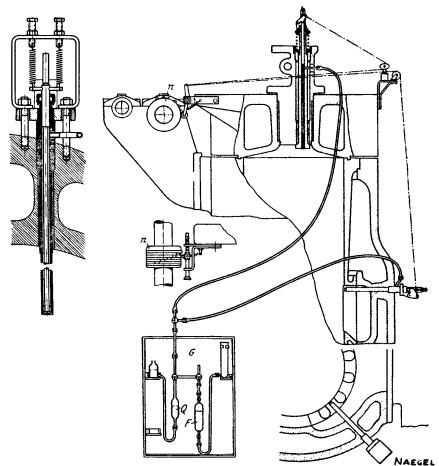
Fig. 16-8. Test Arrangement with Details for Taking Gas Samples from a Sulzer Engine. (Naegel, A., "Dieselmaschine der Gegenwart" *VDI Zeitschr.*, 67, 733, 1923.)
