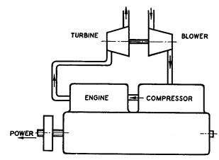
Fig. 15-2. Two-Stage Supercharging. Turbine-driven blower constitutes the first stage and engine-driven compressor the second stage of air compressor.
