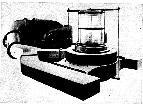
Fig. 16-10. Sass's Outfit for Testing the Scavenging in a Transparent Cylinder. (F. Sass, Kompressorlose Dieselmaschinen. Copyright, 1929, by Julius Springer in Berlin.)
