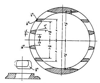
Fig. 8-4. Section through Exhaust Ports of Fairbanks-Morse Opposed-Piston Diesel Engine. (By permission of Fairbanks-Morse Company.)
