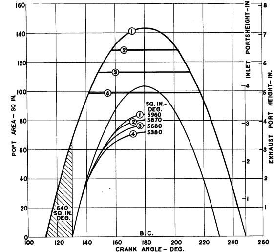
Fig. 14-5. Reduced Port Area Diagrams with Shortened Exhaust Ports. Combined width of inlet ports 20% in. Combined width of exhaust ports 19¾ in.
