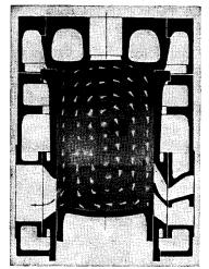
Fig. 5-6. High Scavenge with an Air Swirl in Counterclockwise Direction.
