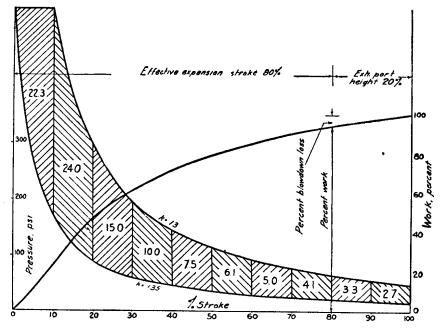
Fig. 10-3. Work-Area of Theoretical Indicator Diagram Reduced by Blowdown Loss. Compression ratio 15:1.
