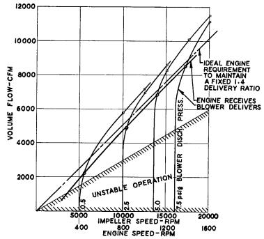
Fig. 11-19. Co-action of Engine and Centrifugal Blower.
