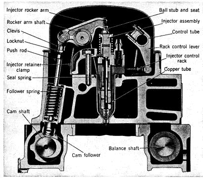
Fig. 17-8. Cylinder Head, Transverse Section.
