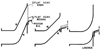
Fig. 5-1, 5-2, 5-3. Duct Shapes for Inlet Ports. Fig. 5-1 produces flat scavenge during almost the entire scavenging period, Fig. 5-2 only near the bottom of the piston stroke, while Fig. 5-3 is free from flat scavenge during the entire piston stroke. The crosses indicate locations of air stream separation.
