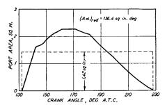
Fig. 9-17. Reduced Time-Area Diagram of General Motors Poppet Exhaust Valve Engine. 4½ in. bore, 5 in. stroke.
