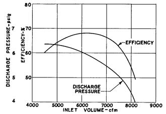
Fig. 11-18. Adiabatic Efficiency of Centrifugal Blower.
