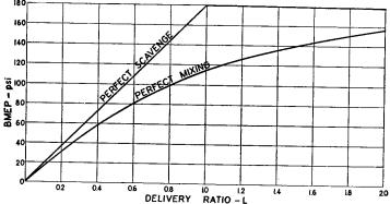
Fig. 4-3. BMEP vs Delivery Ratio at Zero Excess Air. f = 0.4 lb per bhp-hr,  $r_{th} = 14.5$ .
