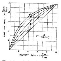
Fig. 3-2. Perfect Scavenge. Air contained in vs air delivered to cylinder in terms of displacement volume.
