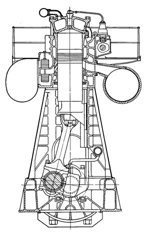
Fig. 17-30. Transverse Longitudinal Section of Nordberg Engine.
