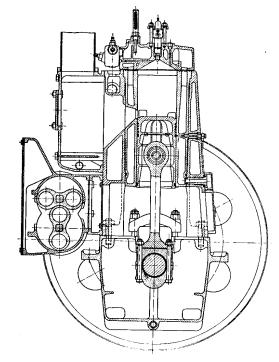
Fig. 12-14. Buckan 6.9 in. × 8.6 in., 600 Rpm Engine with Large Expansion Chamber.
