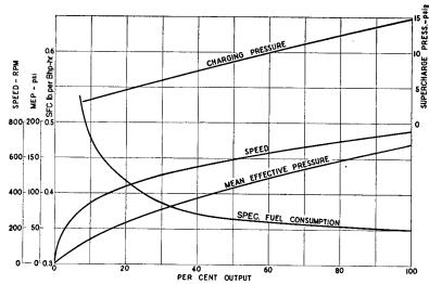
Fig. 15-6. Performance of Sulzer Supercharged Opposed-Piston Engine. Plotted against output when working according to propeller load.
