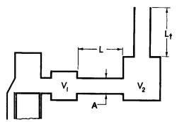
Fig. 12-7. Exhaust System Including a Relatively Small Expansion Chamber.
