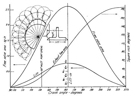
Fig. 8-6. Exhaust Valve Lift, Valve, and Time-Area in General Motors Model 71 Engine. Valve area computed square to the flow.
