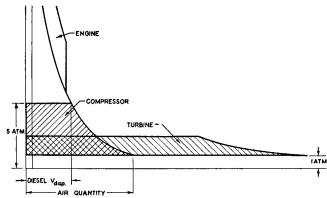
Fig. 15-9. Ideal Indicator Diagram of Power-Gas Process. Engine charged to 5 atm. Compressor work area and engine work area theoretically equal. Upper part of diagram not shown.
