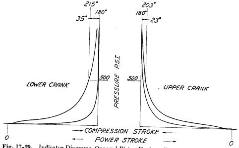
Fig. 17-29. Indicator Diagrams, Opposed-Piston Engine. Ten cylinders, 1600 hp, 720 RPM.
