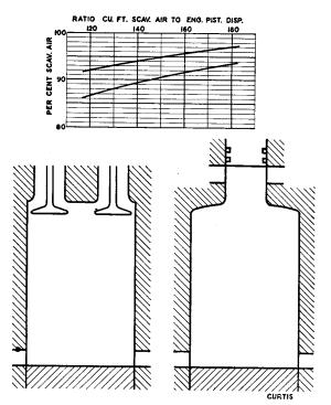
Fig. 16-15. Results with Uniflow Design. Upper curve, no exhaust elbows or hood; lower curve, exhaust hood.
