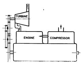
Fig. 15-5. Directly Coupled Reciprocating Compressor and Geared Exhaust Turbine.
