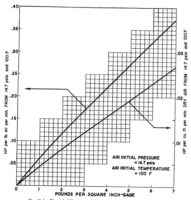
Fig. 11-1. Theoretical Horsepower Requirements for Adiabatic Compression.
