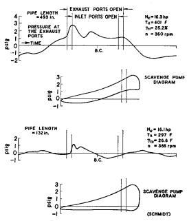
Fig. 12-5. Pressures at Exhaust Ports and in Crankcase. Top diagram shows pressures at ports with exhaust pipe 493 in. long; second diagram shows corresponding crankcase pressures; third diagram shows pressures at ports with exhaust pipe 132 in. long; bottom diagram shows corresponding crankcase pressures. (Th. Schmidt, "Schwingungen in Auspuffleitungen von Verbrennungsmotoren," VDI Dieselmaschinen VI, 79, 1936.)
