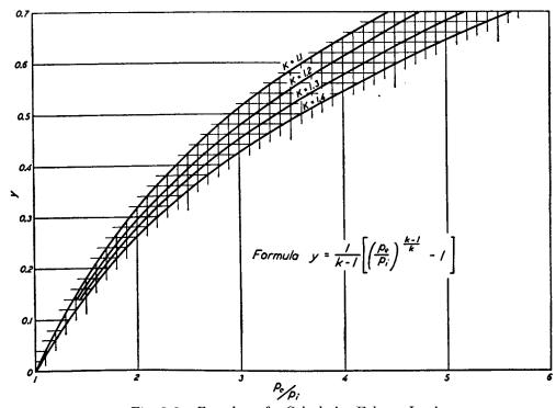
Fig. 8-3. Function y for Calculating Exhaust Lead.
