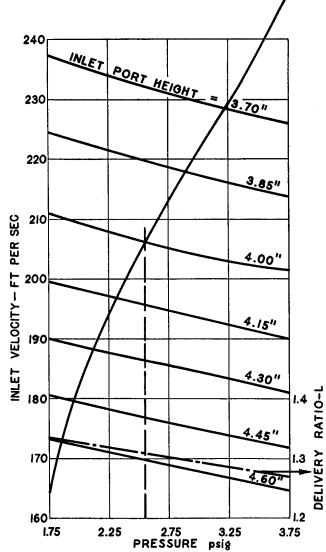
Fig. 14-4. Inlet Velocities vs. Scavenge Pressure.
