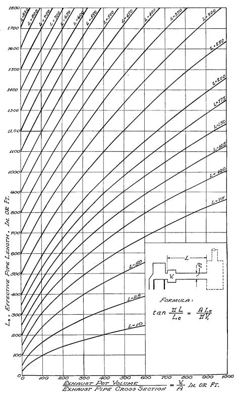
Fig. 12-4. Chart Showing the Equivalent Pipe Lengths for a Frequently Used Exhaust System.
