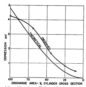
Fig. 13-3. Effect of Size of Opening on Kadenacy Effect. Chamber pressure 5 atmospheres.
