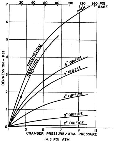
Fig. 13-2. Geyer's Theory Applied to Penn State Experiments.
