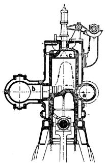
Fig. 7-7. Engine with Simple Port Scavenge. 14.6 in. bore, 20.1 in. stroke, 200 rpm. (Löffler-Riedler, Oelmaschinen. Copyright by Julius Springer, 1916.)
