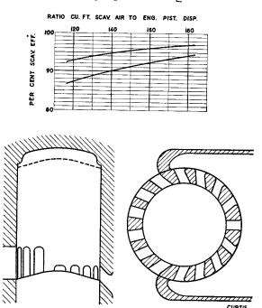
Fig. 16-14. Results of Model Tests on Curtis-Type Loop Scavenging. Lower curve with exhaust hood, upper curve without hood.
