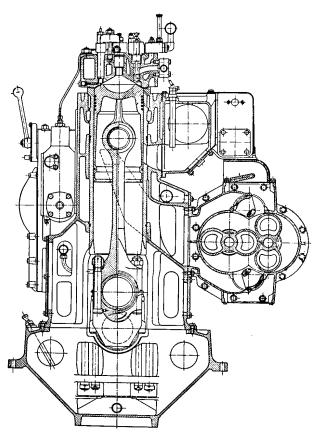
Fig. 11-26. Engine with Liberal Air Chest. Deutz 9.5 in. bore, 13.4 in. stroke, 500 rpm.
