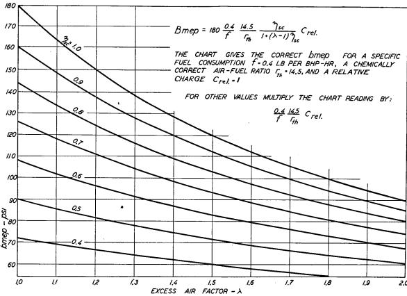
Fig. 4-1. Relation Between Excess Air Factor and Brake Mean Effective Pressure. This chart covers both four-stroke and two-stroke cycle engines at any load.
