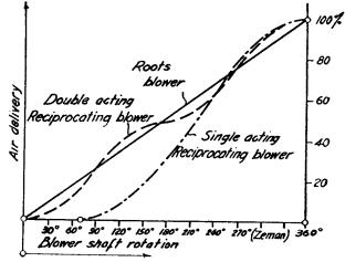
Fig. 11-23. Air Delivery of Roots Blower and Singleand Double-Acting Reciprocating Blowers. (Zeman, Zweitakt-Dieselmaschine, Springer, Vienna. Copyright, 1935, by Julius Springer.)
