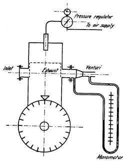
Fig. 16-26. Arrangement to Check Port Timing of an Engine.
