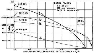
Fig. 12-23. Convertible Exhaust Energy in a Turbine.
