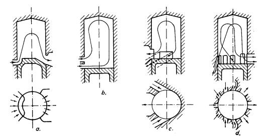
Fig. 2-5. Methods of Scavenging. a. Cross scavenging; b. Loop scavenging, M.A.N. type; c. Loop scavenging, Schnuerle type; d. Loop scavenging, Curtis type.
