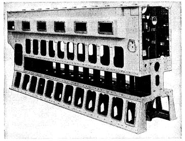
Fig. 17-19. Welded Cylinder Block of Opposed-Piston Engine.
