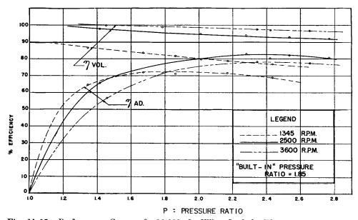
Fig. 11-15. Performance Curves of a 10,000 cfm Elliott-Lysholm Blower. (By permission of the Elliott Company from W. A. Wilson and J. Crocker, "Fundamentals of the Elliott-Lysholm Compressor," ASME Paper 45-A-45, 1945.)
