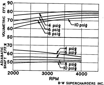
Fig. 11-10. Effect of Speed and Discharge Pressure on the Performance of a Roots-Type Blower. (By permission of B-W Superchargers, Inc.)
