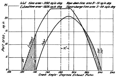
Fig. 9-11. Porting Diagram, Fairbanks-Morse Opposed-Piston Engine.
