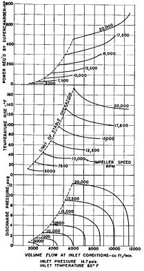
Fig. 11-17. Characteristic Curves of a Centrifugal Blower.
