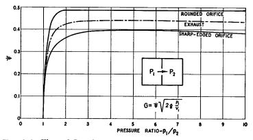
Fig. 8-8. Flow of Gas through an Orifice. Exhaust ports are considered midway between sharp-edged and rounded orifices.
