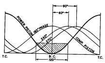
Fig. 11-4. Motion of Power Piston and Compressor Piston. Three phase angles are shown, 180°, 240°, and 270° between the power and compressor pistons.
