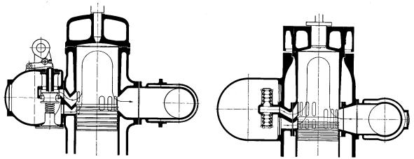
Fig. 9-7. Mechanically Actuated Supercharge Valve in Inlet Duct. (By permission of Sulzer Bros.)
