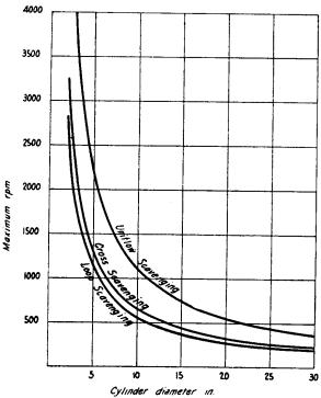
Fig. 10-1. Practical Speed Limits for Two-Stroke Cycle Engines.
