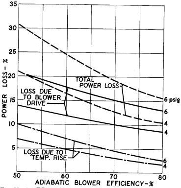
Fig. 11-22. Effect of Blower Efficiency on Engine Power with 4 and 6 psig Scavenge Pressure. Engine gross brep is assumed to be 80 psi.
