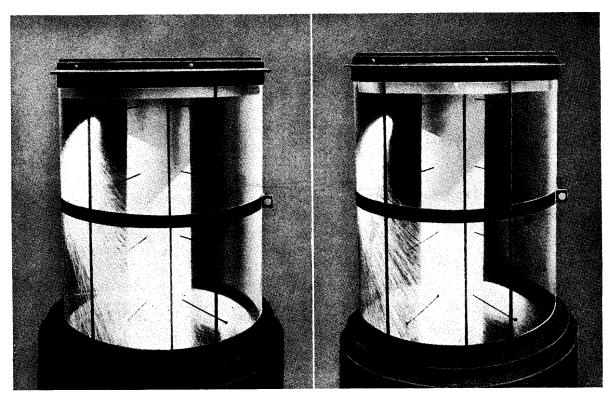
Fig. 16-11. Scavenging Test in a Full Scale Glass Cylinder. (F. Sass, Kompressorlose Dieselmaschinen. Copyright, 1929, by Julius Springer in Berlin.)
