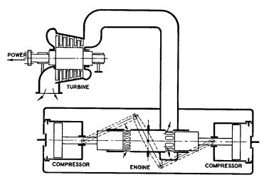
Fig. 15-10. Free-Piston Hot-Gas Generator Turbine Power Plant.
