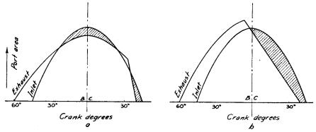
Fig. 9-1. Porting Diagrams with Supercharge. Diagrams a and b have equal timings and time-areas, yet b shows better supercharge.
