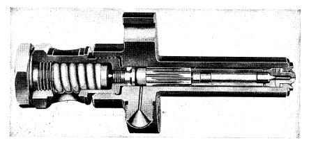
Fig. 17-23. Injection Nozzle, Opposed-Piston Engine.
