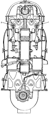
Fig. 7-8. Fairbanks-Morse Opposed Piston Engine. 8 in. bore, 10 + 10 in. stroke, 720 rpm. (By permission of Fairbanks-Morse & Co.)
