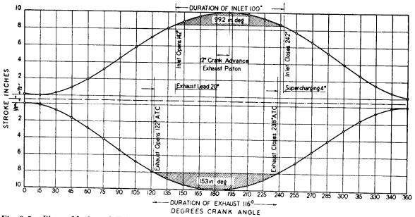
Fig. 8-5. Piston Motion of Fairbanks-Morse Opposed-Piston Engine. This represents the final porting adopted after compromise described in Section 10.10.
