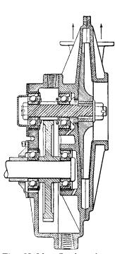
Fig. 11-16. Section through Single-Stage Centrifugal Blower.
