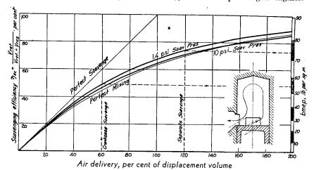
Fig. 5-9. Scavenging Efficiency of Loop Scavenging. Scale on the right shows bmep attainable with 60% excess air, 100% relative charge and 0.5 lb per hp-hr fuel consumption. 70% of the bmep reading represents fair output for symmetrically scavenged engines and 100% for supercharged engines.
