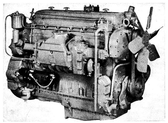
Fig. 17-1. General Motors 6-71 Engine.
