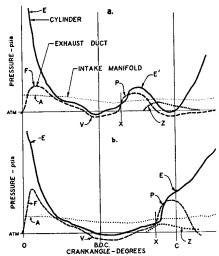
Fig. 12-19. Exhaust Pulse Supercharging Weak-Spring Diagrams. (H. D. Carter, "The Loop Scavenged Diesel Engine," *Proc. Inst. M. E.*, 154, No. 4, 1946.)
