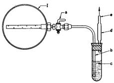
Fig. 16-7. Arrangement Used to Withdraw a Sample Through the Van Slyke-Cullen Urea Apparatus. I — Inlet air duct. a. Sampling tube stopcock. b. Aeration tube. c. Test tube containing sulfuric acid solution. d. Trap to separate any entrained liquid. e. Outlet tube to gas flowmeter. (Penn State Diesel Laboratory.)
