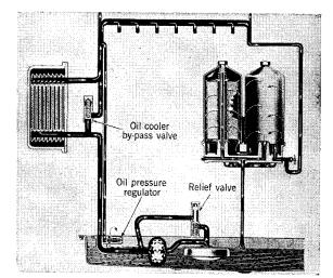
Fig. 17-11. Schematic Lubrication Diagram. Showing path of oil through system having single pressure pump, strainer, cooler, cleanable element filter, and single sump oil pan.
