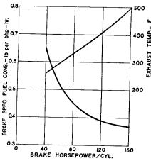
Fig. 17-27. Performance of Fairbanks-Morse Opposed-Piston Engine at 720 RPM.
