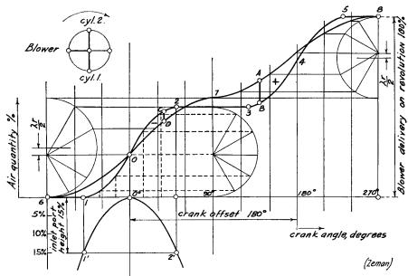
Fig. 11-25. Quantity of Air Delivered into (Line 6-7-8), and Drawn from (Line 1-2-3-4-5-8), the Receiver of a Two-Cylinder Engine with Double-Acting Compressor. (Zeman, Zweitakt-Dieselmaschine, Springer, Vienna. Copyright, 1935, by Julius Springer.)
