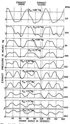
Fig. 16-25. Exhaust Pressure Fluctuations from a GM-71 Engine (Lovett), (Penn State Diesel Laboratory.)
