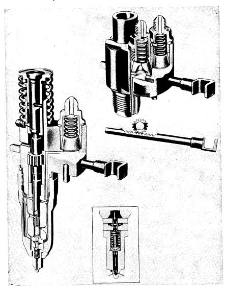
Fig. 17-10. Fuel Injector Assembly.
