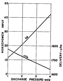
Fig. 14-2. Roots Blower Performance at 1100 Rpm.
