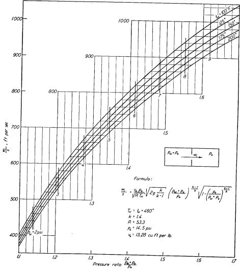
Fig. 7-2. Chart to Determine Mean Velocities. To obtain the mean velocity, multiply the reading on the vertical scale by the estimated scavenge factor which may be taken from Table 7-1.
