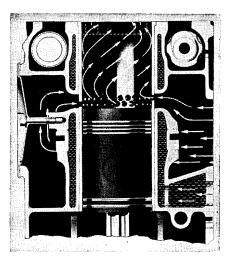
**Fig. 17-4.** Section of Cylinder Block Showing Air and Water Passages.
