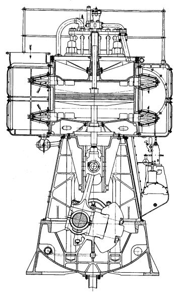
Fig. 11-2. Large Reciprocating Blower. (By permission of Nordberg Manufacturing Company.)
