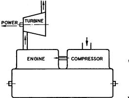
Fig. 15-8. Hot-Gas Generator-Turbine Power Plant. Engine and compressor directconnected, turbine free on exhaust line.
