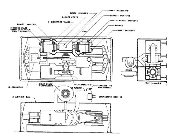
Fig. 15-11. Semifree-Piston Hot-Gas Generator. Two cylinders in tandem with crosshead and synchronizing crankshaft in between.
