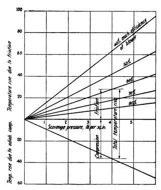
Fig. 11-21. Air Temperature Rise in Blower or Compressor. Example shows that for 4 psig scavenge pressure at 60 per cent blower efficiency the total temperature rise is 67 F.
