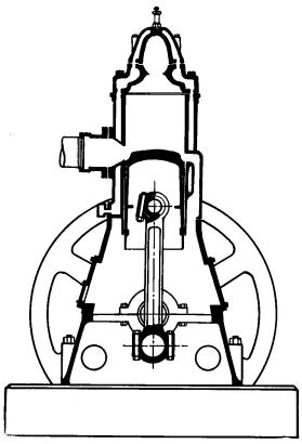
Fig. 7-12. Venn-Severin Crankcase-Scavenged Engine. 10½ in. bore, 12 in. stroke, 425 rpm. (By permission of Venn-Severin Machine Co.)
