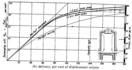
Fig. 5-10. Scavenging Efficiency of Uniflow Scavenging. Scale on the right shows brep attainable with 60% excess air, 100% relative charge and 0.5 lb per hp-hr fuel consumption.
