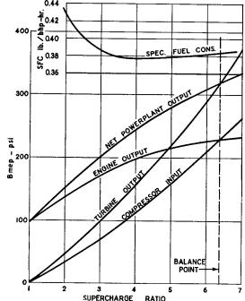
Fig. 15-7. Calculated Performance of Compound Power Plant with Geared Exhaust Turbine.
