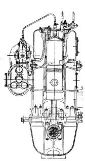
Fig. 12-13. M.A.N. 6.3 in. × 10.2 in., 600 Rpm Engine with Expansion Chamber Surrounding the Cylinders.
