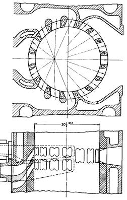
Fig. 6-6. Gothic Ports with Water-Cooled Bridges.
