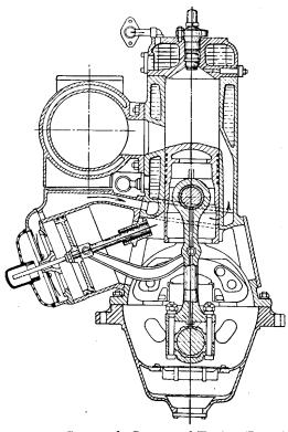
Fig. 2-4. Separately Scavenged Engine (Deutz).
