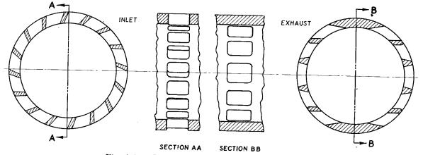
Fig. 6-10. Ports of a Typical Opposed-Piston Engine.
