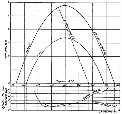
Fig. 9-2. Porting Diagrams and Measured Cylinder Pressures during the Charging Process with (a) Symmetrical and (b) Nonsymmetrical Porting. 4.7 in. bore, 5.9 in. stroke, 700 rpm loop-scavenged engine developing (a) 67.5 and (b) 86 psi bmep respectively. The supercharge was produced by a rotary valve in the exhaust port.
