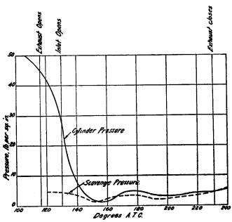
Fig. 16-17. Weak-Spring Diagram of an Engine with Insufficient Exhaust Lead.
