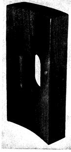
Fig. 6-4. Photograph of Gothic Exhaust Port with Rounded Side Edges.
