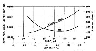
Fig. 13-8. Specific Fuel Consumption and Exhaust Temperatures of Petter Superscavenge Engine.
