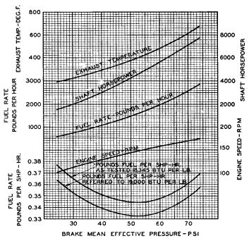
Fig. 17-35. Performance of Nordberg Engine.
