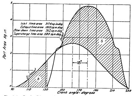
Fig. 9-9. Porting Diagram, General Motors Poppet Exhaust Valve Engine.
