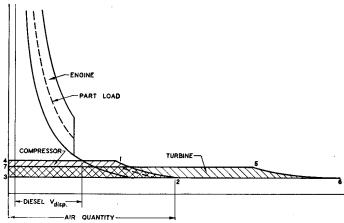
Fig. 15-4. Ideal Indicator Diagram of a Two-Stroke Cycle Diesel Engine Turbocharged to 2 atmospheres (14.7 psig). Upper part of diagram not shown.
