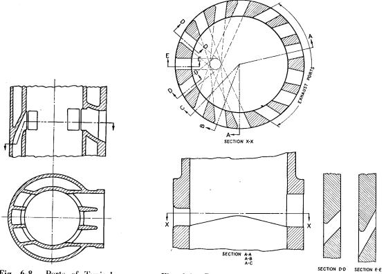
Fig. 6-8. Ports of Typical Cross-Scavenged Engine.
