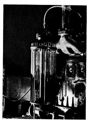
Fig. 16-23. Penn State Rotary-Valve Low-Pressure Indicator. (Penn State Diesel Laboratory.)
