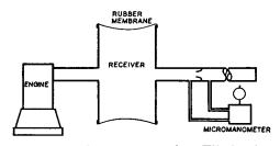
Fig. 16-1. Arrangement for Eliminating Pulsations in Air Flow.
