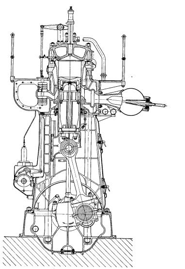
Fig. 9-12. Nordberg Reciprocating Blower Scavenged Engine with Sulzer Type Supercharge Valve (Crosshead Type). 21 in. bore 31 in. stroke, 225 rpm.
