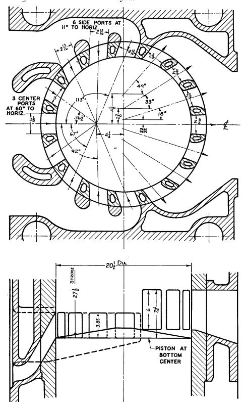
Fig. 14-3. Tentative Layout of Cylinder Block and Liner.
