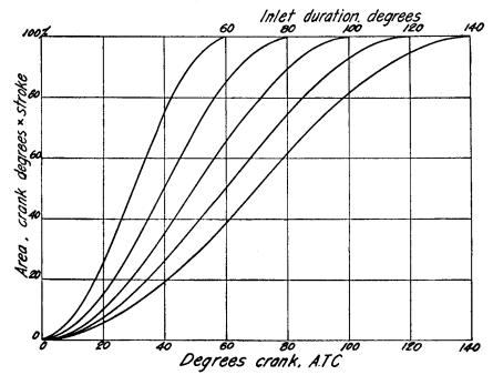
Fig. 11-24. Air Delivery from Receiver into Cylinder with Various Inlet Durations. Piston controlled quadrangular ports and connecting rod-crank ratio of 4.5:1.
