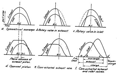
Fig. 6-1. Porting Diagrams of Various Scavenging Arrangements. Uncovered port area vs crank rotation.
