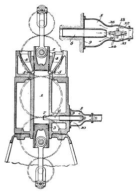
Fig. 13-14. U. S. Patent No. 2,168,528, M. Kadenacy. Means to prevent a too early return of the exhaust gas column that would reach the cylinder when the charging process is still in progress.
