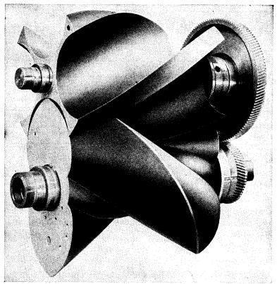
Fig. 11-14. Whitfield Blower with the Rotors in Mesh and Housing Removed. (By permission of J. E. Whitfield Company.)
