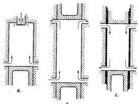
Fig. 2-6. Uniflow Scavenging. a. Poppet valve; 13. Uniflow, slide valve, crankcase-scavenged. b. Opposed piston; c. Sleeve valve.
