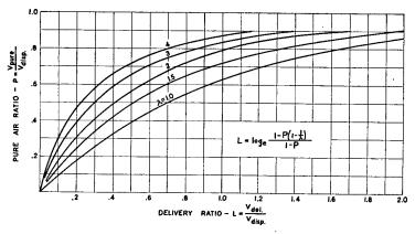
Fig. 3-3. Perfect Mixing. Air contained in vs air delivered to cylinder in units of displacement volume.
