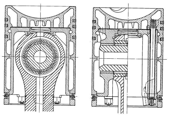
Fig. 17-21. Piston, Opposed-Piston Engine.
