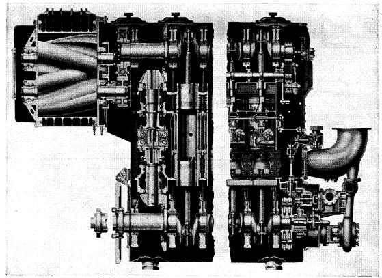
Fig. 17-17. Longitudinal Cross Section. Opposed-Piston Engine.
