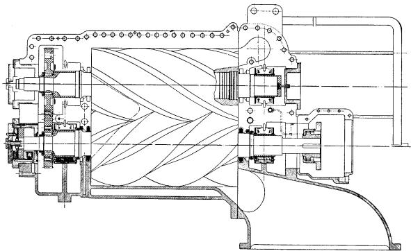
Fig. 11-13. Elliott-Lysholm Blower. (By permission of the Elliott Company from W. A. Wilson and J. Crocker, "Fundamentals of the Elliott-Lysholm Compressor," ASME Paper 45-A-45, 1945.)
