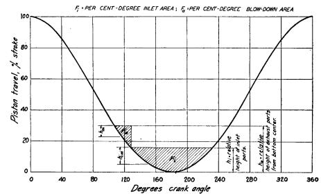
Fig. 7-4. Piston Travel vs Crank Rotation for Connecting Rod-Crank Ratio of 4.5:1.  $F_i$  = Per cent-degree inlet area;  $F_a$  = Per cent-degree blowdown area.
