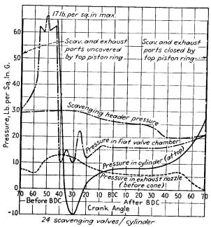
Fig. 16-16. Weak-Spring Diagram of an Engine with Sufficient Exhaust Lead. (By permission of Nordberg Mfg. Co.)
