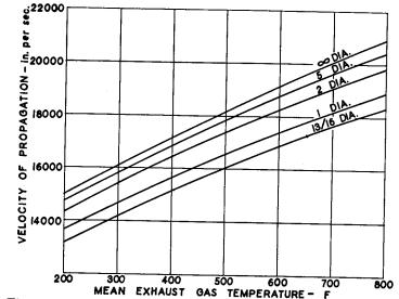
Fig. 12-2. Variation of Propagation Velocity of Pressure Waves in Pipes of Various Diameters.
