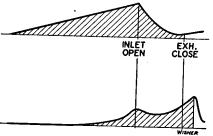
Fig. 11-3. Evolution of the Scavenge Pressure. Top: Rotary blower. Bottom: Reciprocating blower. (R. Wisner, High Speed Two-Stroke Compression-Ignition Engine. The Institute of Automobile Engineers, June, 1944.)
