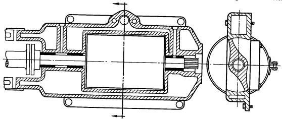
Fig. 9-4. Cooper-Bessemer Supercharge Valve in the Exhaust. (By permission of Cooper-Bessemer Corp.)
