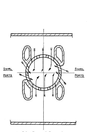
Fig. 13-5. Inlet Ports of Petter Superscavenge Engine. In this section through cylinder and liner arrows indicate the believed air flow causing rotation of charge.
