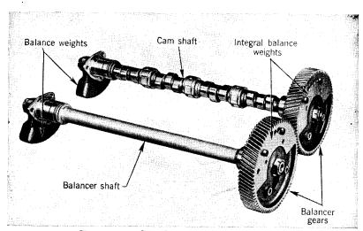
Fig. 17-9. Camshaft and Balancer Shaft.
