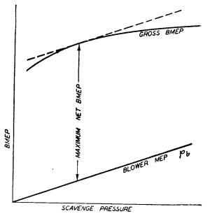
Fig. 7-6. Showing the Principle of Determining the Scavenge Pressure that Gives Maximum Net Bmep.
