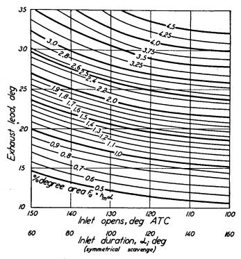
Fig. 8-1. Exhaust Lead with Piston Controlled Ports. Connecting rod-crank ratio 4.5:1. (The inlet duration scale is not valid for nonsymmetrical engines.)
