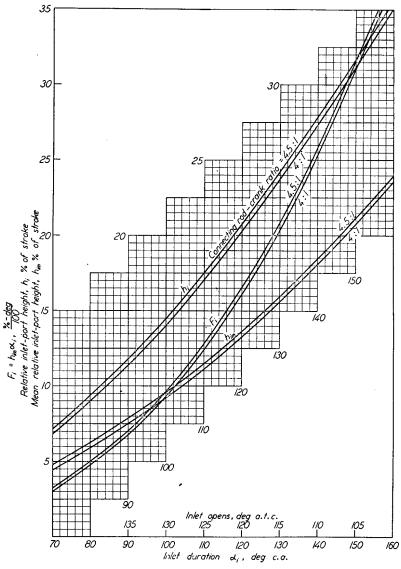
Fig. 7-5. Port Height and Per Cent-Degrees vs Inlet Duration for 4.5:1 and 4:1 Connecting Rod-Crank Ratios. As  $h_i$  and  $h_{im}$  are expressed in % stroke, the chart readings must be divided by 100 before they are used.  $F_i$  readings are 1/100 of the %-deg. values, therefore they are to be used unchanged. By substituting  $\alpha_e$  for  $\alpha_i$ ,  $h_e$  for  $h_i$  and  $F_e$  for  $F_i$ , the curves are applicable to exhaust ports as well.
