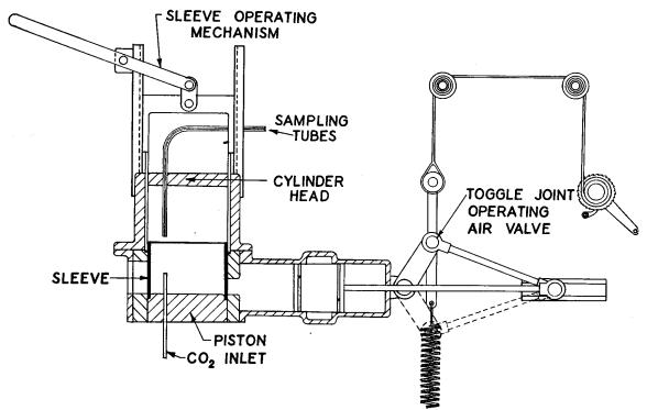
Fig. 16-12. Curtis' Testing Apparatus for Determining the Efficiency of Scavenging.
