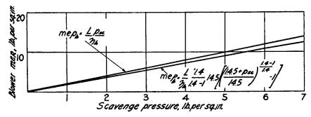
Fig. 11-20. Blower mep for a Delivery Ratio of L=1.4 and a Blown Efficiency of  $\eta_b=0.7$ . Lower curve is based on formula for adiabatic compression, upper curve on simplified formula.
