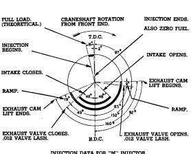
Fig. 17-14. Timing Diagram with "M" Injectors.
