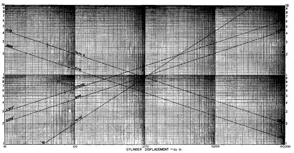
Fig. 18-1. Principal Data for Various Size Cylinders with a Stroke-Bore Ratio of 1.4 and a Bmep of 66 psi. These data correspond to a piston speed of 1260 fpm and result in a power output of 1.26 hp per sq. in. piston area.
