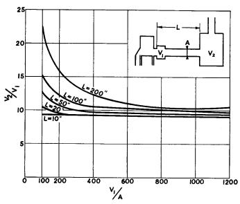
Fig. 12-6. Chart Showing Selection of Size of Expansion Chambers. For given value of  $V_1/A$  and L, ordinate shows minimum value of  $V_2/V_1$  so that period differs no more than 5 per cent from the value obtained with  $V_2/A = \infty$ .
