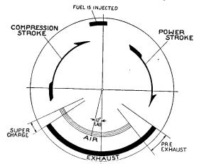
Fig. 17-28. Timing Diagram, Opposed-Piston Engine.
