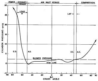
Fig. 13-9. Weak-Spring Indicator Diagram of Petter Superscavenge Engine. (B. M. Dale, "Recent Development in Medium-Speed Two-Cycle Oil Engines," *Motor Ship*, 25, No. 300, Jan., 1945.)
