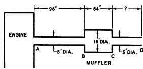
Fig. 12-10. Arrangement of Exhaust System.
