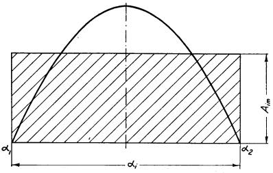
Fig. 7-3. Calculation of Inlet Port Dimensions. The formula is  $A_{im}\alpha_i = \frac{L}{2w_i}V_{disp}n; w_i$  is to be taken from Fig. 7-2.
