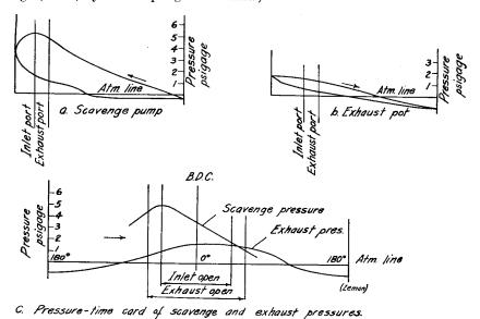
Fig. 16-19. Weak-Spring Diagrams with Improperly Functioning Exhaust System. 12.6 in. bore, 14.6 in. stoke, 310 rpm; exhaust pipe 5.9 in. dia., 356 in. long; exhaust pot 8.7 cu. ft. (J. Zeman, Zweitakt Dieselmaschinen. Copyright, 1935, by Julius Springer in Vienna.)
