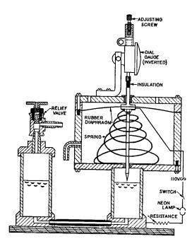
Fig. 16-5. Penn State Differential Micromanometer.
