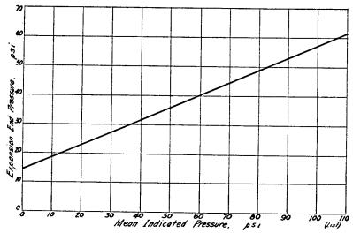
Fig. 8-2. Relation between Expansion End Pressure and Mean Indicated Pressure.
