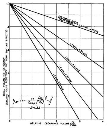
Fig. 11-7. Volumetric Efficiency of Reciprocating Air Compressor vs. Clearance Volume. Deduct 5-10% slippage from ideal volumetric efficiency.
