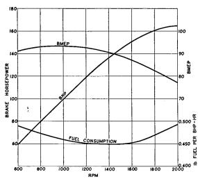
Fig. 17-15. Performance Characteristics of General Motors 6-71 Engine with "M" Injectors.
