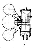
Fig. 9-3. Rotary Valve in Exhaust Hamilton-M.A.N. double acting engine. (By permission of Lima-Hamilton Corp.)
