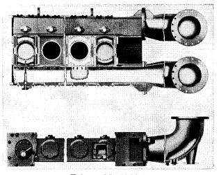
Fig. 17-20. Exhaust Manifold Arrangement.
