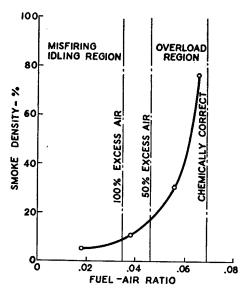
Fig. 16-30. Smoke Density against Load, "Normal" Engine. (Penn State Diesel Laboratory.)
