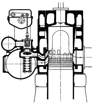
Fig. 15-1. Sulzer Method of Supercharging with Separate High-Pressure Air. (Courtesy Sulzer.)
