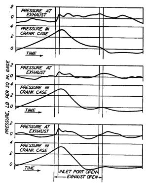
Fig. 12-1. Effect of Tuning on Pressure Fluctuations at Exhaust Ports and in Crankcase of Crankcase-Scavenged Engine during one Cycle. Top diagram shows poor tuning; thermal efficiency was 22.2 per cent. Middle diagram is slightly better, with thermal efficiency of 24.5 per cent. Bottom diagram shows good tuning; thermal efficiency rose to 25.2 per cent. (Th. Schmidt, "Schwingungen in Auspuffleitungen von Verbrennungsmotoren," VDI Dieselmaschinen VI, 79, 1936.)
