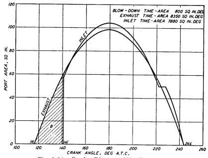
Fig. 9-14. Porting Diagram of Nordberg Engine.
