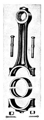
Fig. 17-5. Connecting Rod Details.
