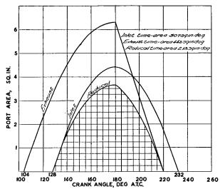
Fig. 9-15. Porting Diagram. 4.5 in. bore, 6 in. stroke, 1800 rpm.
