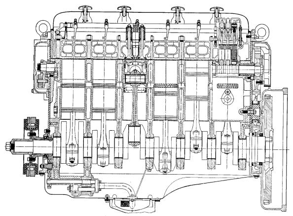
Fig. 17-2. Longitudinal Cross Section GM 6-71 Engine.
