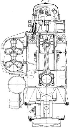
Fig. 7-10. General Motors Model 71 Engine. 4<sup>1</sup>/<sub>4</sub> in. bore, 5 in. stroke, 2000 rpm. (By permission of General Motors Corp.)
