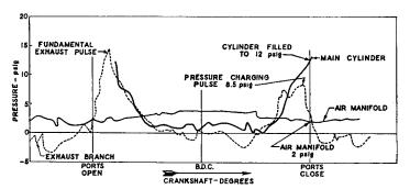
Fig. 12-20. Optimum Exhaust Pulse Supercharging.  $10\frac{1}{2}$  in. bore,  $13\frac{1}{2}$  in. stroke, three-cylinder engine, 330 bhp. Cathode ray oscillogram taken from cylinder No. 1. 76 psi bmep at 500 rpm. (H. D. Carter, "The Loop Scavenged Diesel Engine," *Proc. Inst. M. E.*, 154, No. 4, 1946.)
