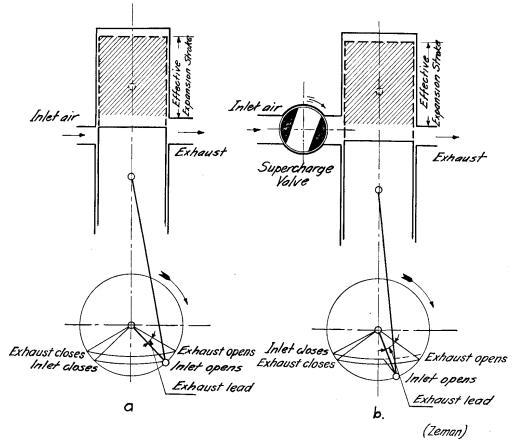
Fig. 2-1. a. Symmetrical and b. Unsymmetrical Scavenging. Note the early exhaust opening and late inlet closing made possible with supercharge valve. (J. Zeman, Zweitakt Dieselmaschinen, Springer, 1935. Copyright, 1935 by Julius Springer in Vienna.)
