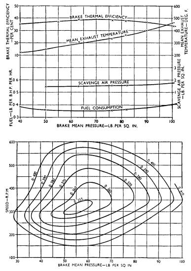
Fig. 12-18. Performance of Crossley-Carter Engine. 10½ in. bore, 13½ in. stroke, oil cooled pistons. (H. D. Carter, "The Loop Scavenged Diesel Engine," *Proc. Inst. M. E.*, 154, No. 4, 1946.)
