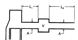
Fig. 12-8. Exhaust System With an Exhaust Pot in the Middle of the Exhaust Pipe.
