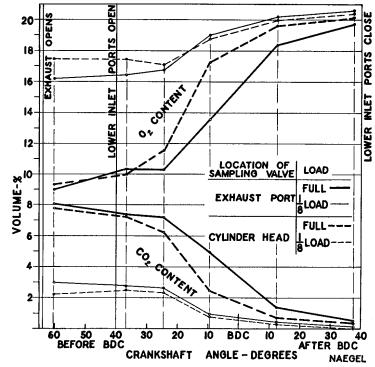
Fig. 16-9. Sample Gas Analysis from a 1600 Hp Sulzer Engine. (Naegel, A., "Dieselmaschine der Gegenwart," VDI Zeitschr., 67, 733, 1923.)
