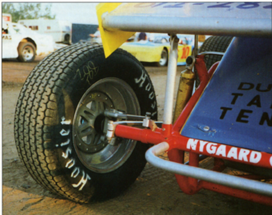
Sprint cars racing on dirt typically do not use right front brakes. The team monitors the front tyre sizes (note the circumference dimension chalked on the tyre wall), but front stagger does not affect left:right front brake bias as it would with two front brakes.
