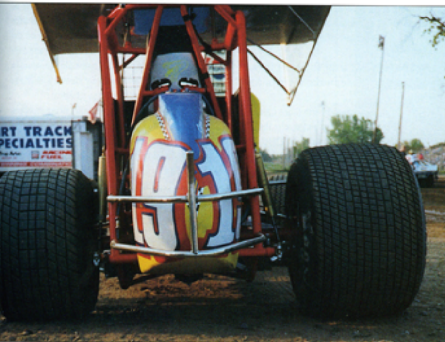
This Sprint car displays large front:rear disparity in tyre sizes. Together with ample rear aerodynamic downforce, this allows the car to run ferocious rear stagger (below), without becoming excessively 'loose'.
