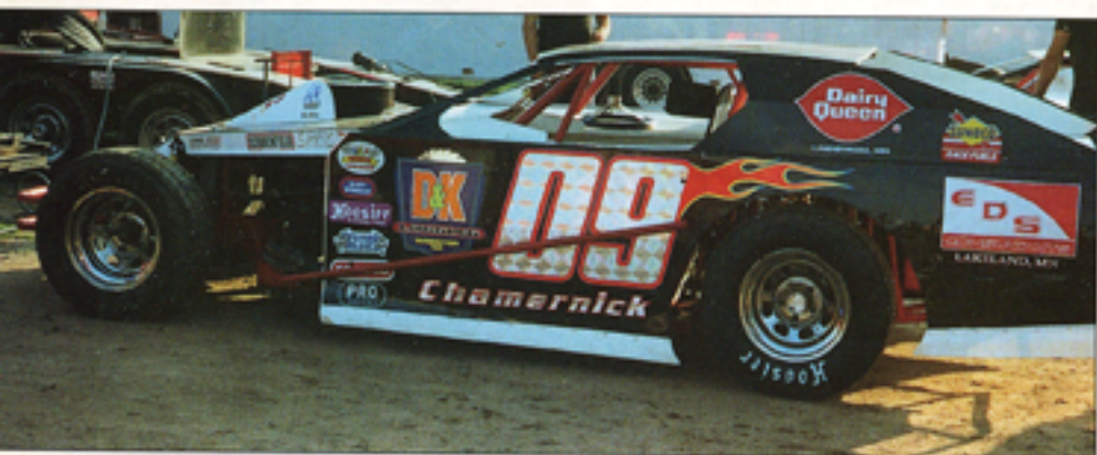
This Dirt Modified runs under WISSOTA rules, which allow generous engine set-back, yet impose an identical tyre size limit front and rear. These cars cannot use large amounts of rear tyre stagger without becoming prohibitively 'loose'.
