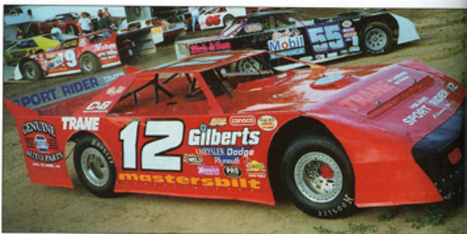
WISSOTA Late Models (car 12) and Super Stocks (car 55) have identical front and rear tyre size limits. Late Models are allowed much wider tyres than Modifieds, but less engine set-back.
