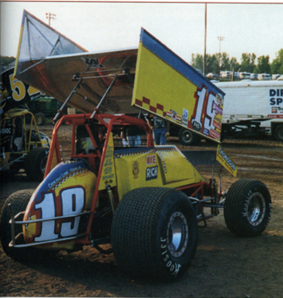
This Sprint car displays large front:rear disparity in tyre sizes. Together with ample rear aerodynamic downforce, this allows the car to run ferocious rear stagger (below), without becoming excessively 'loose'.
