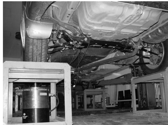
Figure 7. Modal test set-up for the rear suspension system.
