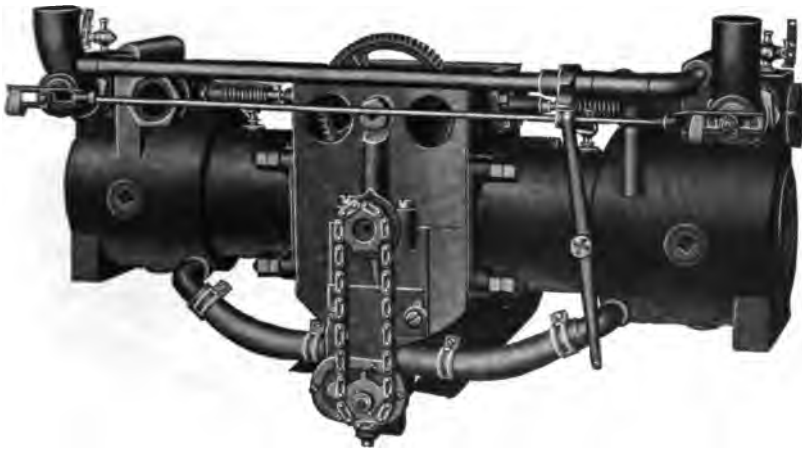
FIG. 247.—Stevens-Duryea Motor—Pump Side. The spur-gear water force pump is driven by sprockets and chain from the crank shaft. The charge admission is throttled by moving the small sliding rod connected to the vertical lever seen at the right. This small rod, just below the mixture tube, reaching horizontally from one cylinder to the other, carries valve lift limiting wedges at each end, which permit greater or less rise of the automatic inlet valves, according to the wedge rod adjustment. The crank case cap is secured by wing nuts, and can be very quickly removed and replaced.
