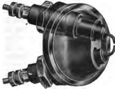
FIG. 219.—Double Spark Plug used on the Cadillac Carriage. Unlike other plugs, the secondary circuit is carried by visible leads, and is not grounded at any point. Superior sparking qualities are claimed, and, as seems evident, fouling is a more remote danger.
