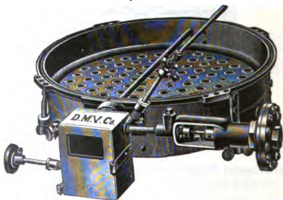
FIG. 441.—The Dayton Burner, showing the Starter Box and Regulator in Position.
