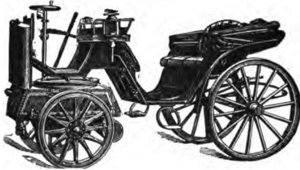
FIG. 58.—The Pretot Fore-Carriage shown attached to a Victoria Carriage. The attachment is on a fifth wheel running on roller bearings, and turning by geared connections with the steering hand wheel.
