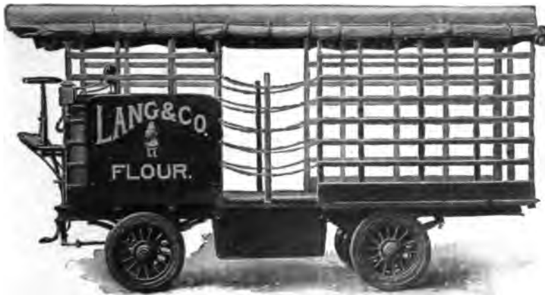
FIG. 340.—Heavy truck of the Vehicle Equipment Co. Carrying capacity, 4 tons; speed, 6 miles per hour; travel radius on one charge of battery, 25 miles.
