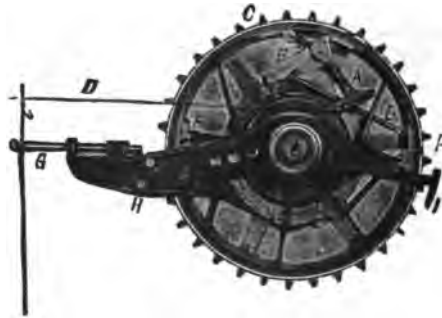
FIG. 126.—The "Duryea" Expanding Brake. The two ends of the metal band are separated by the lever, A, and the adjusting screw, B, which is swiveled to the hinge, C. A forward pull on lever, A, through the chain, pull, indicated by D, causes the two ends of the band to be thrust apart and bear against the inner surface of the sprocket. The extension spring, E, normally holds the band away from this friction surface. The two lugs, F F, attached to a spider hung on the axis of the sprocket, take the braking effort from the bottom of the band more into the line of travel. A framework, indicated at H and I, supports a leather guard covering both the chain and sprocket.
