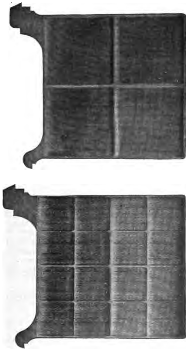
FIG. 373.—Specimen Negative Plate of a Type of the "Gould" Storage Battery, showing the result of "formation" in the changed appearance of the plate surface.
