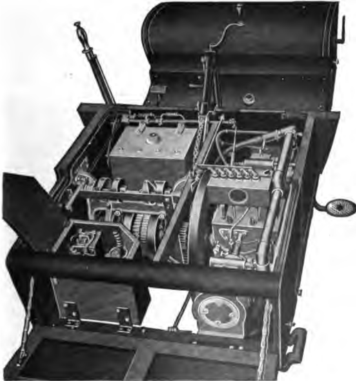
FIG. 321.—Motor and Control Apparatus of the Stevens-Duryea Car. Starting by horizontal crank; steering by upright crank; speed shifting by hand lever at left; throttling by button at end of upright lever.
