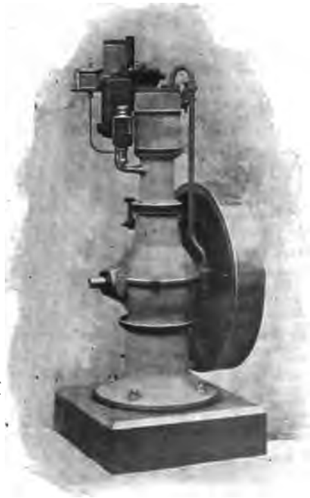
FIG. 141.—A Daimler Single-Cylinder motor intended for Stationary Use. Attached to the head of the water-cooled cylinder are the gasoline chamber and carburetor. The lubricating cup is shown immediately below. The exhaust valve, not shown, is operated by a cam on the secondary shaft, geared to the crank shaft, as may be seen within the fly-wheel. In essential particulars this motor is identical with those used for vehicle propulsion; the method of mounting being, of course, different.
