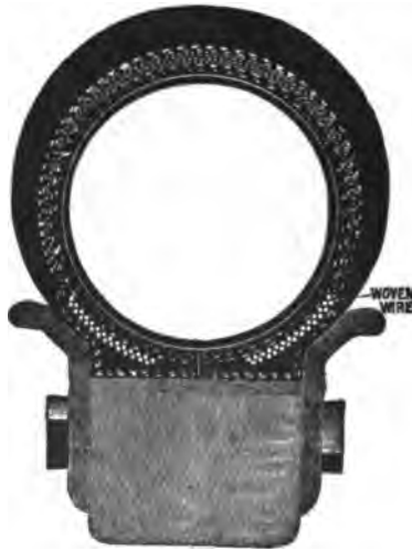
FIG. 104.—The Goodyear Double-Tube Tire. The attachment of this tire is by the strips of wire, woven like a cotton shoestring, which spread apart under the pressure of inflation, thus securing a rigid hold.
