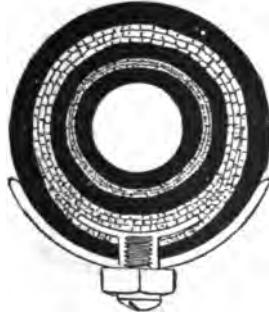
FIG. 99.—The New York E. & P. Single-Tube Tire. The extra thick walls of this tire render puncture less easy, and also provide for a "cushion," or semi-solid, support in case of deflation. The method of attachment by lugs and nuts to a semi-circular channel is one adopted by a large number of other tires, affording a secure hold at the base to safeguard against creeping.
