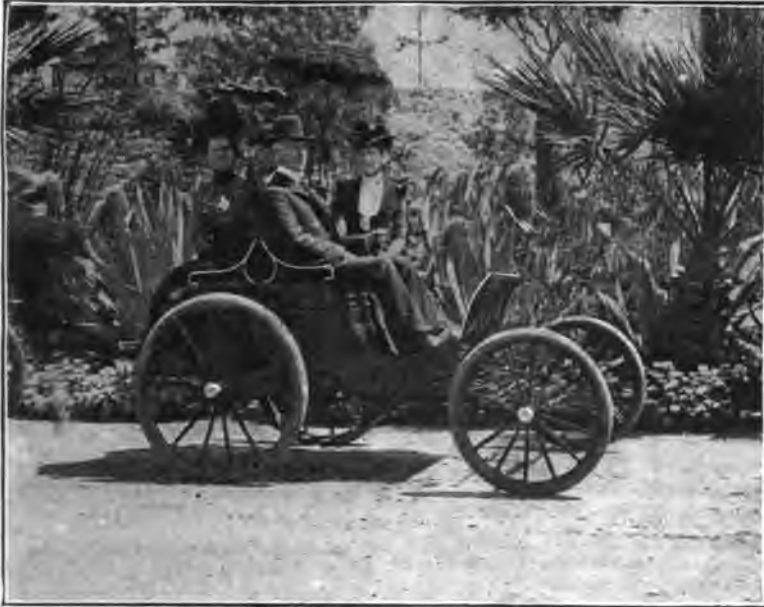
FIG. 68.—Duryea Four-wheeled Trap. This carriage, like all others made by the Duryeas, has no underframe; the strongly built body serving as a frame to which the axles and springs are hung.
