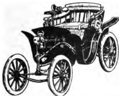
FIG. 31.—Panhard-Levassor Light Two-Passenger Car, having a Swinging Front Axle. The steer wheel pillar carries an arm on its end to which is attached a link bar working a similar arm on the pivot of the axle, as shown.
