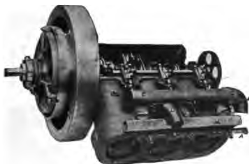
FIG. 250. —The Duryea Three-cylinder 10 1-2 B. H. P. Carriage Motor. A is the throttle slide, by which the gas supply to the three cylinders may be controlled by the combined steering and control lever shown in the last figure; B, single wire connecting anvils of the three sparking plugs in multiple, the other terminal of the circuit being connected to the middle parts of the cylinder; C, the common exhaust tube conveying the burned-out gases to the muffler; D, the pipe conveying air to the jackets of the three cylinders.
