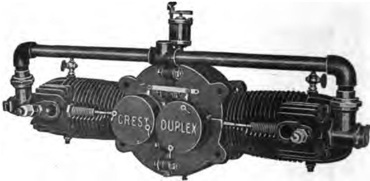
FIG. 148. — "Crest" Double-Opposed Cylinder Gasoline Vehicle Engine, showing radiating ribs for cooling cylinders. The cylinders of this motor are in line, not off-set, as in some makes, the two cranks working on one crank pin. Owing to the method of joining the crank case on its diameter, all the working parts may be readily reached by unscrewing four bolts. Among the special features of this motor are the relief valve, which opens, hence interrupting operation as the wagon coasts down hill, and the automatic cut out for the battery circuit which operates when the engine is at a standstill.
