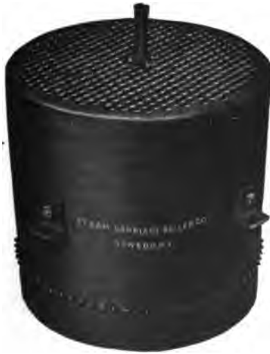
FIG. 401.—Small Carriage Boiler made from a seamless steel pressing, the lower tube plate being flanged over and riveted in, as indicated at the base of the figure, this being the only seam in the structure.
