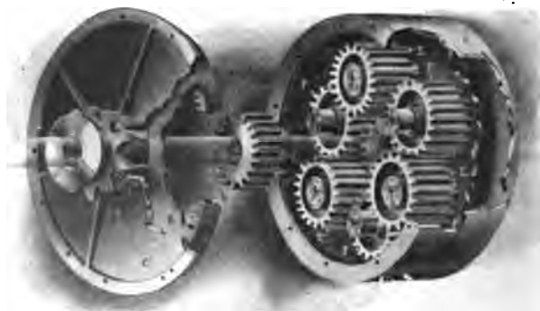
FIG. 325.—Diagram of the Cadillac Transmission, giving two forward speeds and one reverse.
