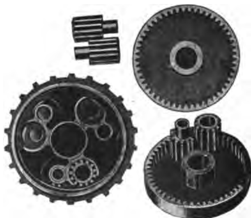
FIG. 27. —Another form of Spur Balance Gear. The action is the same as in Fig. 26, except that the inner ends of the divided axle carry internal gear wheels, each of which meshes with one pinion of each pair.
