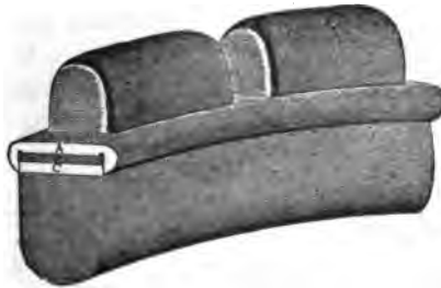
FIG. 95.—Solid Rubber "Sectional Tire," having the tread divided into a number of tooth-like sections, all attached in one piece to the rubber base, as shown, in order to give greater distortion endwise under load, thus allowing of considerable cushion effect. It has been claimed that the construction permits of real resiliency.
