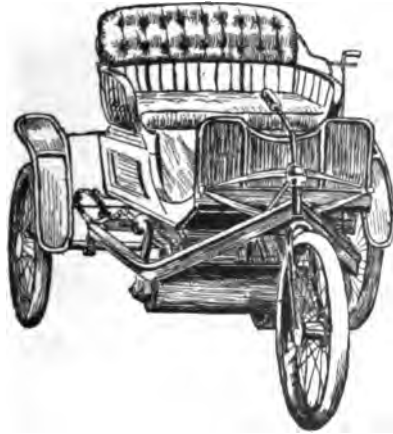
FIG. 70.—The Knox Three-wheeled Gasoline Phaeton, showing angle iron underframe, three-point support and steering connections.
