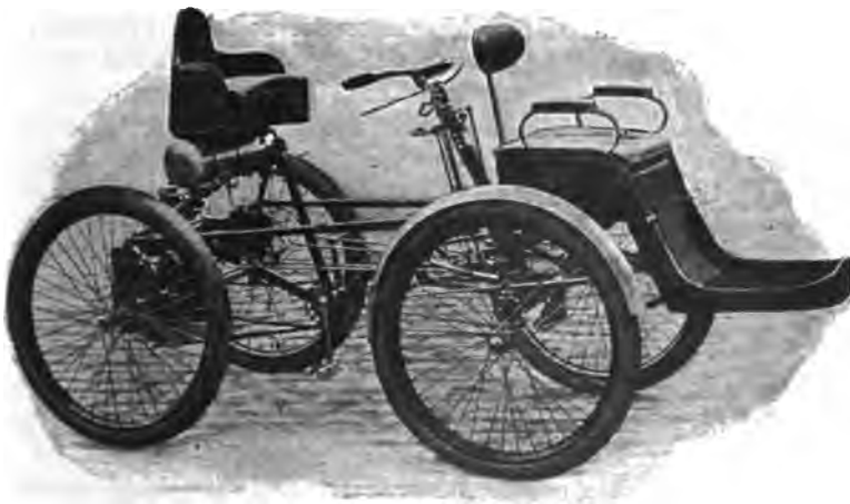
FIG. 118.—A De Dion Gasoline Quadricycle, for carrying two persons. This vehicle consists of a motor tricycle whose forward wheel has been removed in order to allow attachment to the two-wheeled fore-carriage, as shown.
