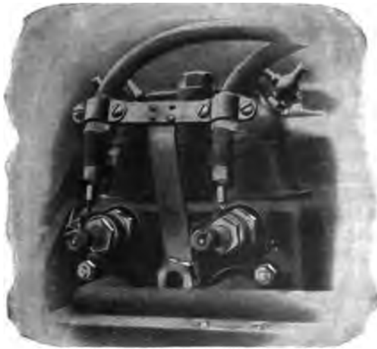
FIG. 208.—Outside Spark Gap in the form of Chains, as applied on the Riker-Locomobile engine.
