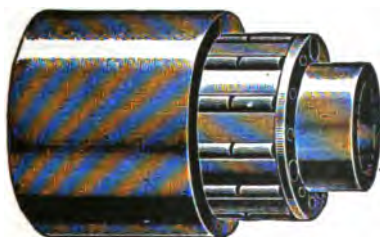
FIG. 129. —Roller Bearings Enclosed in a Retaining Cage. The bearings are hung to the two end pieces of the cage, being separated by stationary pieces of metal. The inner tube is the rotating axle; the outer, the axle box.
