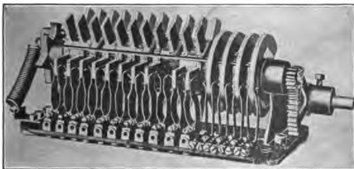
FIG. 367.—A Typical Electrical Vehicle Controller, or Circuit-changing Switch. The circuit terminals of battery and motors are shown at the jack-springs, which are arranged to be engaged by the fins on the periphery of the controller-cylinder. The connections within the controller between the fins are the same as those shown in Fig. 366, except for the fact that the four rings at the right hand end provide constant voltage connections for use with a shunt motor. The gaps at the rear of the rings show means for cutting out the shunt field at top speed.
