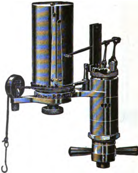
FIG. 385.—A Typical Steam Engine Indicator. It consists of a cylinder, shown at the right, within which works a piston under tension of a helical spring of predetermined strength. The rod attached to the piston carries a pivoted arm which works on the horizontal lever, shown at the top of the cylinder. This lever carries a pencil bearing against the rotatable drum, shown at the left. This drum is so arranged with a spring that it may be rotated by the pull on the attached string. A sheet of paper is wound on the drum and held in place by the spring clips. The steam pressure in the cylinder acting on the spring enables the pencil to mark; the indicator card being traced by the rotative movement of the paper drum.
