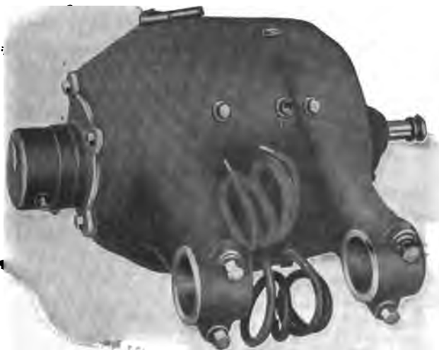
FIG. 344.—General Electric Motor, Designed for Heavy Vehicle Use, with single or double reduction. Capacity, 30 amperes at 85 volts; 800 R. P. M. at full load.
