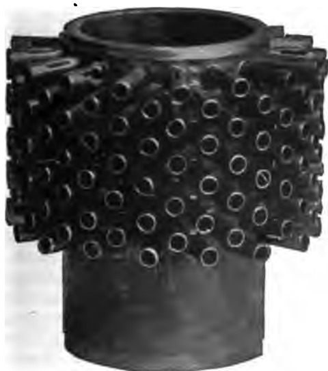
FIG. 153.—Cylinder of the Regas Motor, showing Bunsen tubes let into steel jacket.
