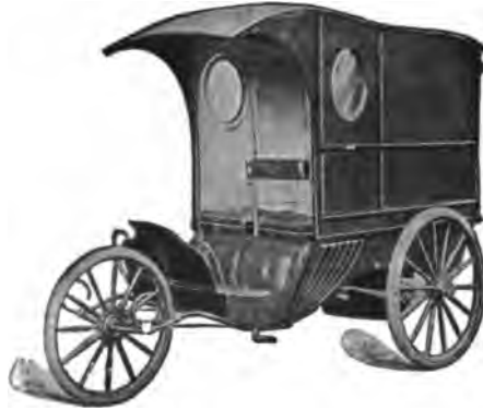
FIG. 71. —Duryea Three-wheeled Delivery Wagon. This wagon is built on the plan shown in Fig. 67.
