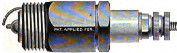
FIG. 211.—“American” Indestructible Sparking Plug. This plug has two essential parts—the shell carrying one electrode, which screws into the metal of the cylinder, and the core composed of mica, through which runs the other terminal, the two being joined together by screw connections as shown. The superior advantages of mica insulation, as claimed by the manufacturers, are that heat has no effect whatever upon it; thus rendering it much more durable than a plug made of porcelain or other substance liable to be affected by heat and allow short-circuiting of the sparking current.
