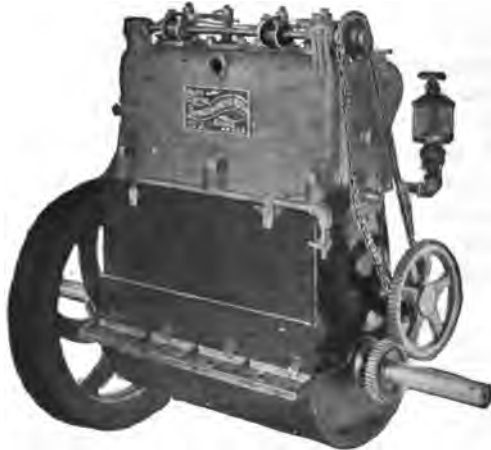
FIG. 162.—Four-Cylinder, 10 H. P. "Buffalo" Gasoline Engine for Motor Vehicle Use. The gearing of this motor renders it non-vibrating, as guaranteed, while, by the "shifting-spark" system of governing, the speed may be varied from 100 to 1,500 R. P. M. without changing the motion of the valves. This is an exceedingly flexible system of governing. The cylinder head is water-jacketed; the firing stroke in the four cylinders follows consecutively, thus securing perfect balance; the inlet valves are positively operated, thus enabling a wide range in adjusting fuel charge ratios. On account of the four-cylinder positive igniters, the engine is very easy to start.
