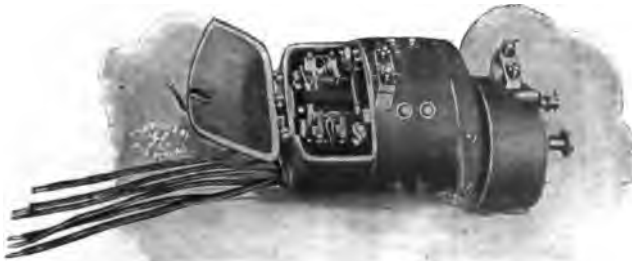
FIG. 342.—Type of General Electric Light Vehicle Motor, with case open, showing commutator and brush apparatus. The pinion end head is arranged for double reduction. Both end heads and gear housing are made of aluminum. Suspension by lugs to body. Capacity, 31\frac{1}{2} amperes at 39 volts; 1,800 R. P. M. at full load.
