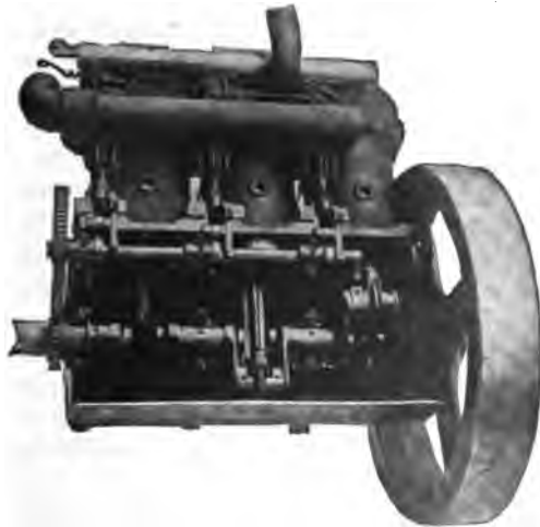
FIG. 161.—The Duryea Three-Cylinder Gasoline Vehicle Engine, with half the crank case sheathing removed, showing cranks, crank shaft, cam shaft, and working parts. The three cylinders have common supply and exhaust tubes; the charge is controlled by a single throttling link, shown at the top, and the igniting circuit has three bridges for the three cylinders
