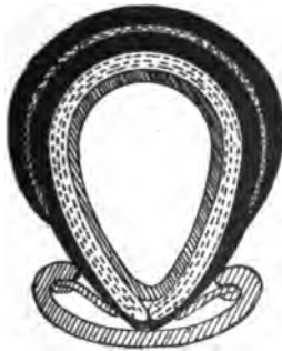
FIG. 103.—The "Grappler" Tire. Instead of endless wires, this tire carries projecting flanges of metal strips at either side of the base, which press against the inner overlapping sides of the channel rim, affording a secure attachment.
