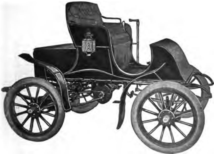
FIG. 355.—Studebaker Electric Runabout, with Chain and Sprocket Connections between Motor hung on the Body and the Rear Axle. The advantage is that the motor is protected from the jars of travel by the springs.
