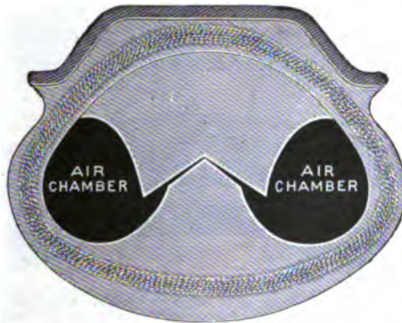
FIG. 105. —The Munger Single-Tube Tire. This view shows the tire deflated, so that the longitudinal rubber buffers come together, thus forming a semi-solid, or cushion tire, and preventing the inconvenient consequences generally following this condition.
