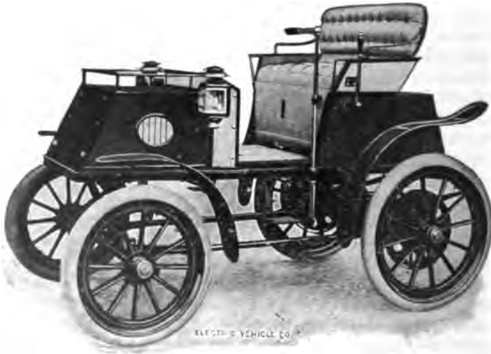
FIG. 336. —“ Columbia ” Electric Runabout. This carriage, weighing about 1,200 pounds, has a traveling radius of about forty miles per full charge of battery, and a maximum speed of thirteen miles per hour.
