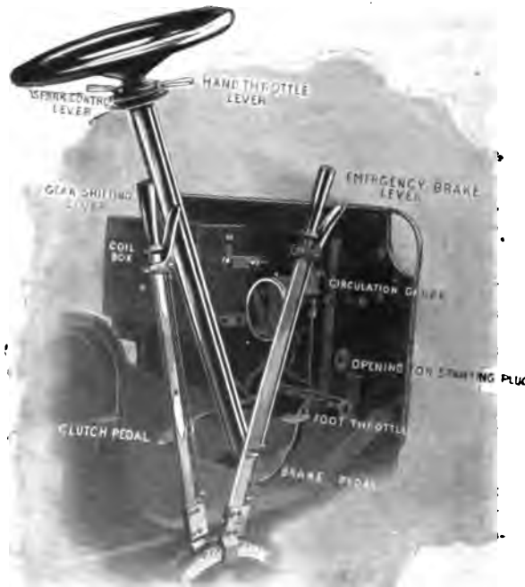
FIG. 290.—Control Levers and Appliances of the Riker Car.
