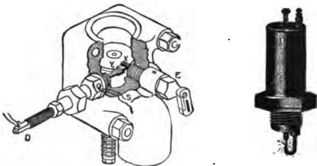
FIG. 189.—Details of a Common Form of Contact for Producing a Wiping Spark. The electrode, X , rotated by the crank, E , as indicated, gives a wiping contact and break at the terminal, Y , which is tipped by a resilient platinum spring. One of the wires forming the circuit is connected at D through the insulated plug screwed into the body of the ignition chamber; the other is connected to the metal of the chamber at the nut, M . The advantage of this form of sparking device is that the constant contact of the electrode keeps the surfaces clean, but at the same time the constant friction produces an immense wear for the same reason. An excellent form of simple make-and-break device is shown in connection with the suction of the Duryea cylinder in a succeeding chapter.
