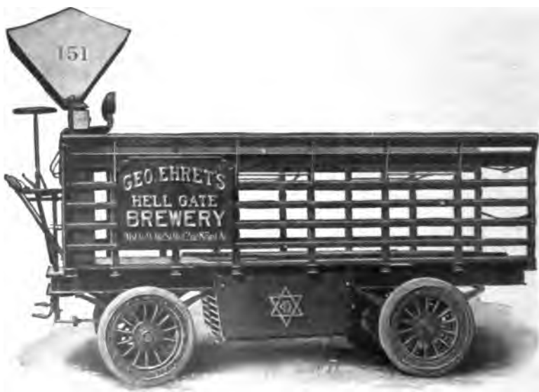
FIG. 357.—Electric Brewery Wagon of the Vehicle Equipment Co. Carrying capacity, 5 tons; speed, 6 miles per hour at full load; travel radius on one charge, 25 miles.
