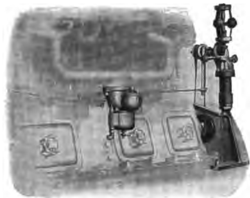
FIG. 66.—Centrifugal governor attached to carburetor.
