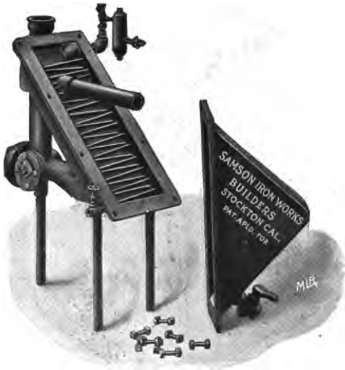
FIG. 318.—The crude-oil generator.
