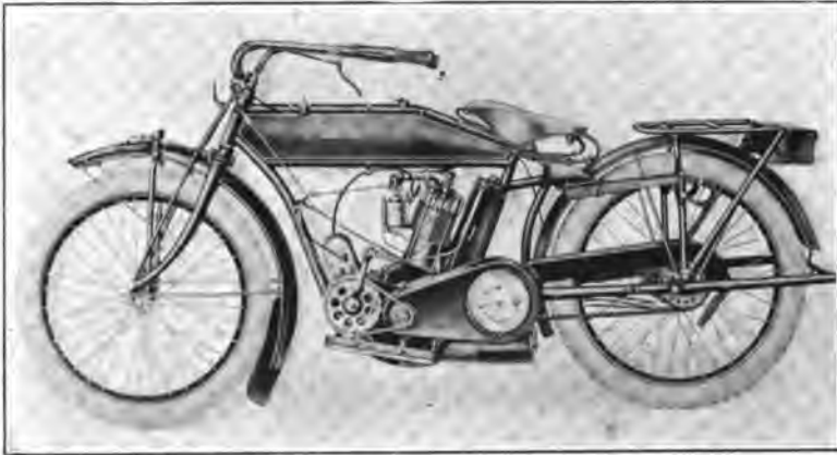
FIG. 395.—Typical single cylinder motorcycle of modern design, incorporating two-speed gear, spring frame, and kick starting arrangement.
