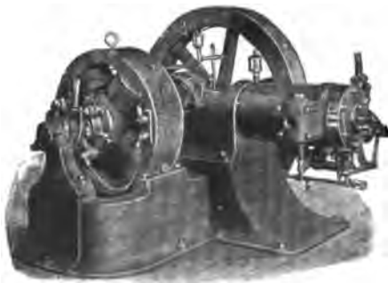
FIG. 219.—Direct-connected engine and generator.
