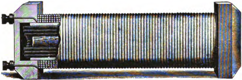
FIG. 75.—Construction of low-tension sparking coil.
