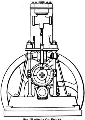
Fig. 121.—SECOR OIL ENGINE. Side Elevation. (Paragraph 239)
