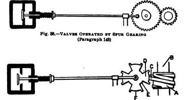
Fig. 39.—Valves Operated by Worm Wheel Cam. (Paragraph 144)
