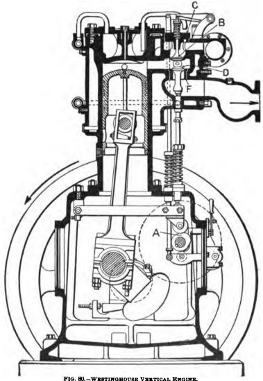
FIG. 80.—WESTINGHOUSE VERTICAL ENGINE. Cross Section through Cylinder and Valve Chembers, (Paragraphs 60, 208.)
