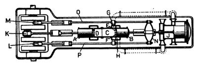
FIG. 104.—OECHELHAUSER TWO-CYCLE ENGINE. Sectional Plan. (Paragraph 222)
