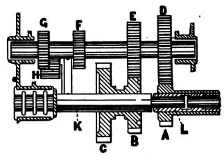
Fig. 153.—Diagram of the Decauville Transmission Grar.
