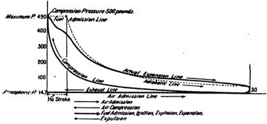
Fig. 26.—Indicator Diagram of Engine; Heating at Constant Temperature.
