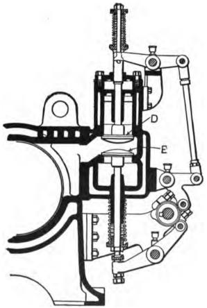
FIG. 87.—BLAISDELL ENGINE. Cross Section through Valve Chambers. (Paragraph 209)
