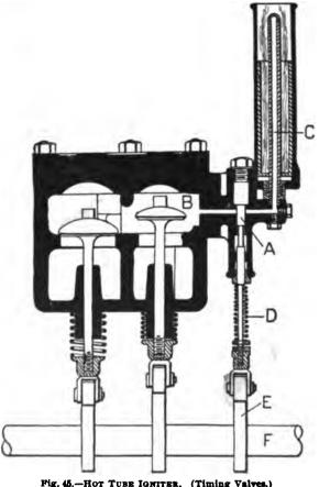
Fig. 45.—Hot Tube Igniter. (Timing Valves.) (Paragraph 158)
