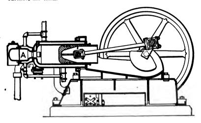
Fig. 116.—HORNSBY-AKROYD OIL ENGINE. Longitudinal Section. (Paragraph 287.)
