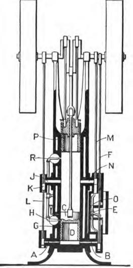
Fig. 99.—RIKER DOUBLE-PISTON TWO-CYCLE ENGINE, (Paragraph 218)
