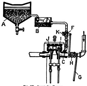
Fig. 120.—Secor Oil Engine, Gravity Feed Arrangement, (Paragraph 239)
