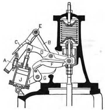
FIG. 85.—NÜRNBERG ENGINE. Gas Valve Mechanism. (Paragraph 208)
