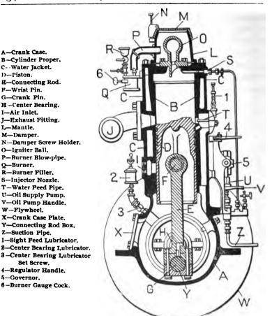
FIG. 131. - MEITZ AND WEISS MARINE ENGINE. Vertical Section through one Cylinder. (Paragraph 246)
