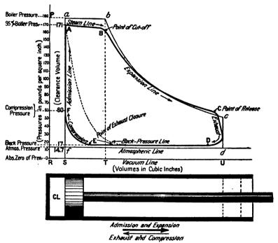
Fig. 20.—Theoretical Diagram of Stram Engine (Paragraphs 80-83)
