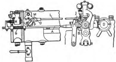
Fig. 63.—WAYNE ENGINE, VALVE GEAR AND GOVERNOR. (Paragraph 196)
