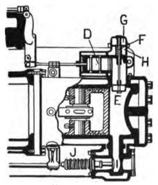
FIG. 72.—BURGER ENGINE. Sectional View of Valve Chambers. (Paragraph 201)
