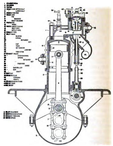
Fig. 147.—Section of Typical Automobile Motor.
