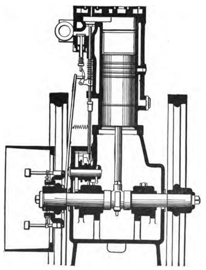
Fig. 78.—NASH ENGINE. Vertical Longitudinal Section. (Paragraph 205.)
