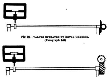
Fig. 87.—VALVES OPERATED BY SPIRAL GEARING. (Paragraph 143)
