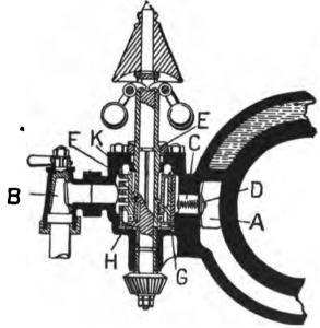
Fig. 48.—CENTRIFUGAL FLY-BALL THROTTLING GOVERNOR. (Paragraph 158)
