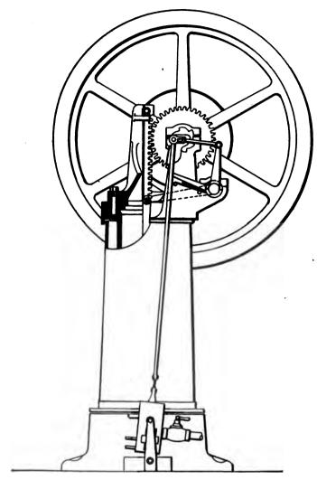
Fig. 3.—Otto-Langen Atmospheric Engine (1862)
