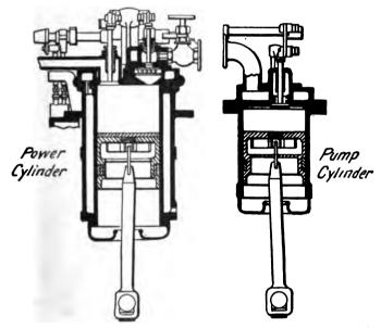
Fig. 5.—Brayton Engine, cross sections through cylinders. (Paragraph 8)
