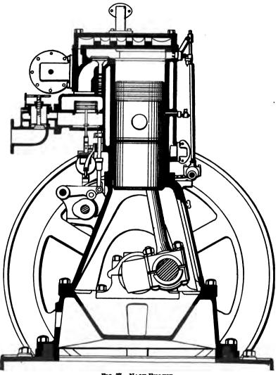
Fig. 77.—NASH ENGINE. Vertical Cross Section. (Paragraph 205.)
