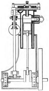
Fig. 7.- OTTO FOUR-CYCLE ENGINE (Paragraph 9.)
