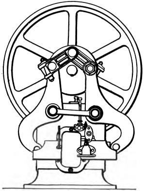
Fig. 97.—Atkinson Differential Engine. Side Elevation. (Paragraph 217)
