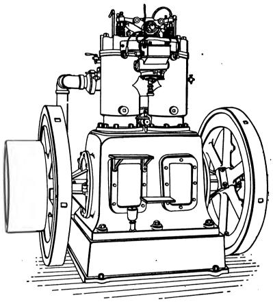
FIG. 81.—MERIAM-ABBOTT ENGINE. Two-Cylinder Unit, 85 Horse-Power. (Paragraph 207)
