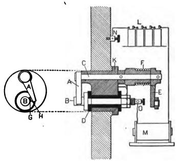
Fig. 46.—HAMMER-BREAK IGNITER. (Paragraph 161)
