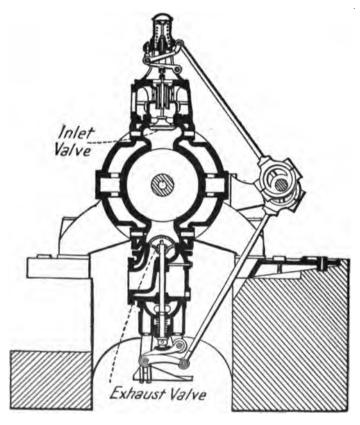
FIG. 84.—NÜRNBERG KNGINE. Section through Valve Chambers, (Paragraph 208.)
