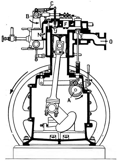
Fig. 9.—FOUR-CYCLE ENGINE (Paragraph 60)
