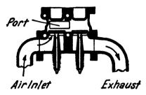
FIG. 117.—HORNSBY-ARROYD ENGINE. Longitudinal Section through Valves. (Paragraph 237.)
