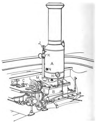
Fig. 128.—Naphtha Engine Installation, (Paragraph 248)
