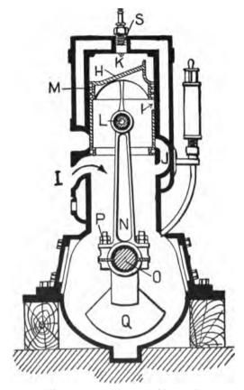
FIG. 128.—FAIRBANES GASOLINE MARINE ENGINE, Vertical Section through one Cylinder, (Paragraph 245)
