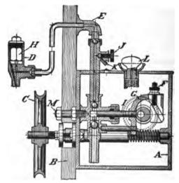
FIG. 145 .- SECTION THROUGH A TYPE OF POWER-DRIVEN OIL PUMP.
