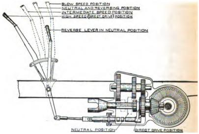
Fig. 154.—Diagram of Control Levers and Transmission of the Packard Car.
