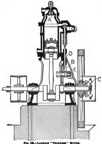
Fig. 109.—LACROIX "PROGRESS" MOTOR, Vertical Section. (Paragraph 229)
