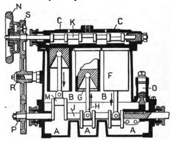
Fig. 184.—Naphtha Engine. Longitudinal Section. (Paragraph 248)
