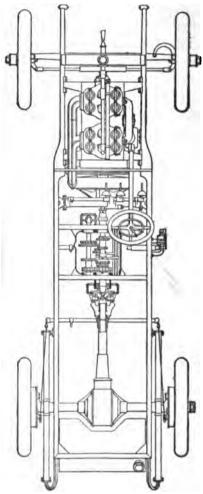
Fig. 149.—Plan of 50 Horse-Power Chassis. (Paragraph 878)
