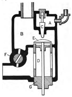
Fig. 111.—Simple Form of Carburetter. (Paragraph 283.)
