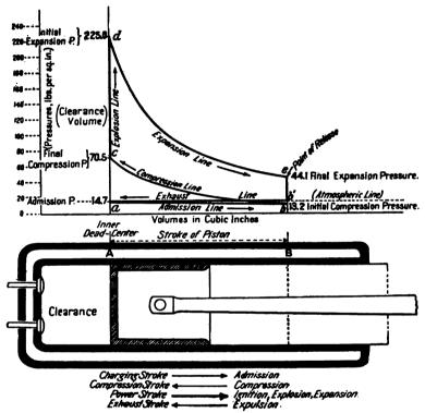
Fig. 21.—Theoretical Indicator Diagram of Gas Engine (Paragraphs 84-85)
