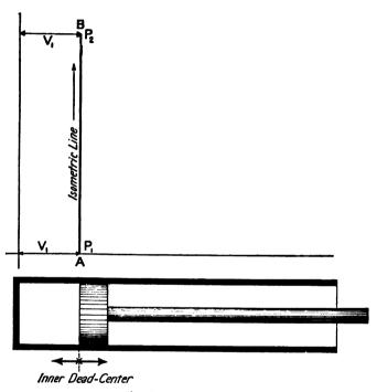
Fig. 17.—ISOMETRIC LINE (Paragraph 74)
