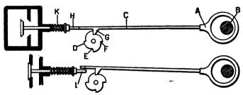
Fig. 40.—VALVE OPERATED BY ECCENTRICS.
