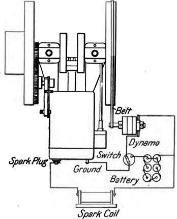
Fig. 49.—WIRING DYMAMO OR MAGNETO FOR MAKE-AND-BREAK IGNITION.
