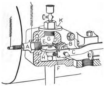
Fig. 47.—WIPE CONTACT IGNITER.
