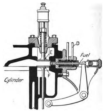
FIG. 119.—AMERICAN DIESEL ENGINE. Section through Fuel, Air, and Exhaust Valves. (Paragraph 238)
