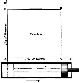
Fig. 12.—PRESSURE VOLUME DIAGRAM (Paragraph 68)
