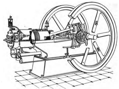
Fig. 61.—WAYNE GAS AND GASOLINE HNGINE. Valve Gear Side, (Paragraph 196)
