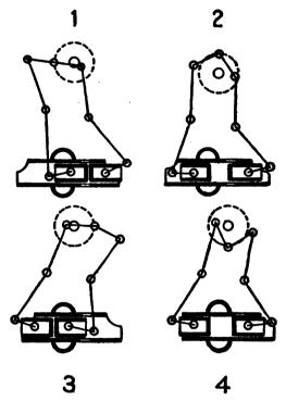
FIG. 98.—ATKINSON DIFFERENTIAL ENGINE.
