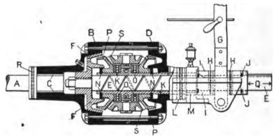
Fig. 122.—Friction Clutch Reversing Gear-(Paragraph 247)
