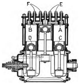
FIG. 108.—ROSER-MAZURIER COMPOUND GAS ENGINE.
