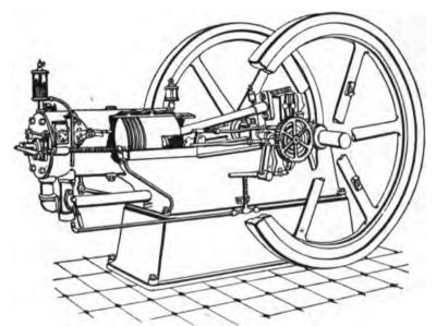
Fig. 61.—WAYNE GAS AND GASOLINE ENGINE. Valve Gear Side. (Paragraph 196)
