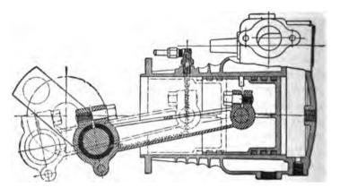
FIG. 144.—HORIZONTAL CYLINDER OILED BY FORCE-FEED OIL DISTRIBUTER.
