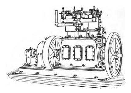
FIG. 79.—WESTINGHOUSE ENGINE. Three-Cylinder Unit, 800 Horse-power. (Paragraph 206.)
