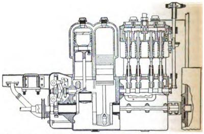
FIG. 150.—PART SECTIONAL ELEVATION OF THE PACKARD FOUR-CYLINDER ENGINE.
