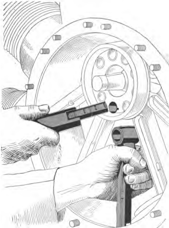
FIG. 93.—Wristpin withdrawn and piston lowered.
