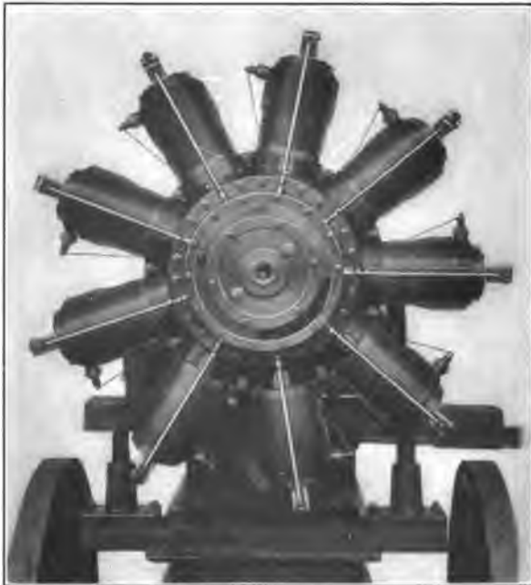
FIG. 86.—Gnome engine in test frame.
