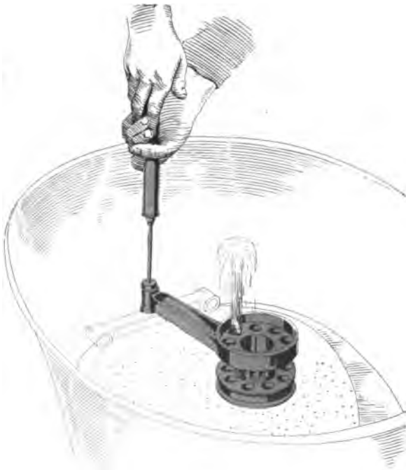
FIG. 98.—Cleaning and washing mother rod.
