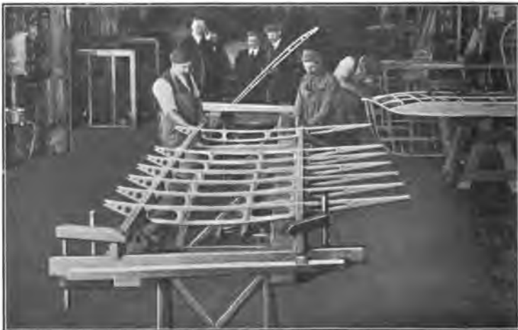
FIG. 131.—Assembling wing with spars.
