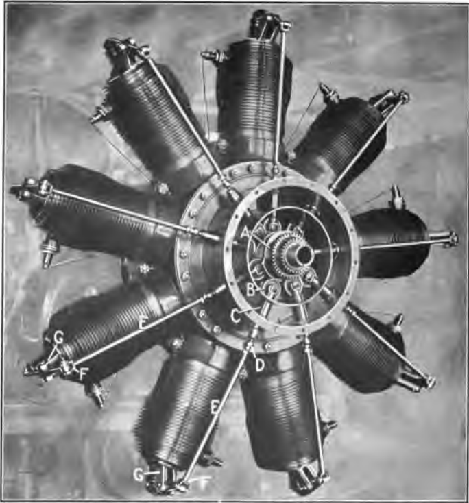
FIG. 88.—Cam action of Gnome engine.
