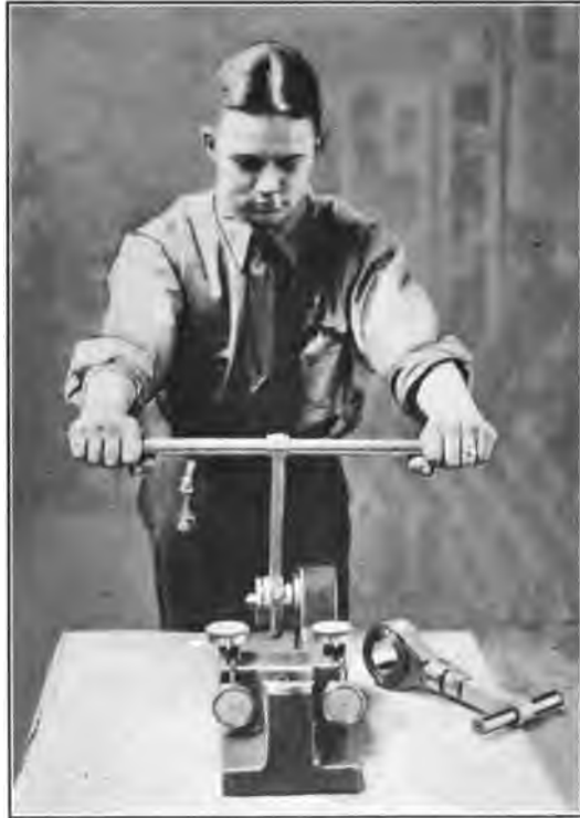
FIG. 64.—Straightening connecting rods.
